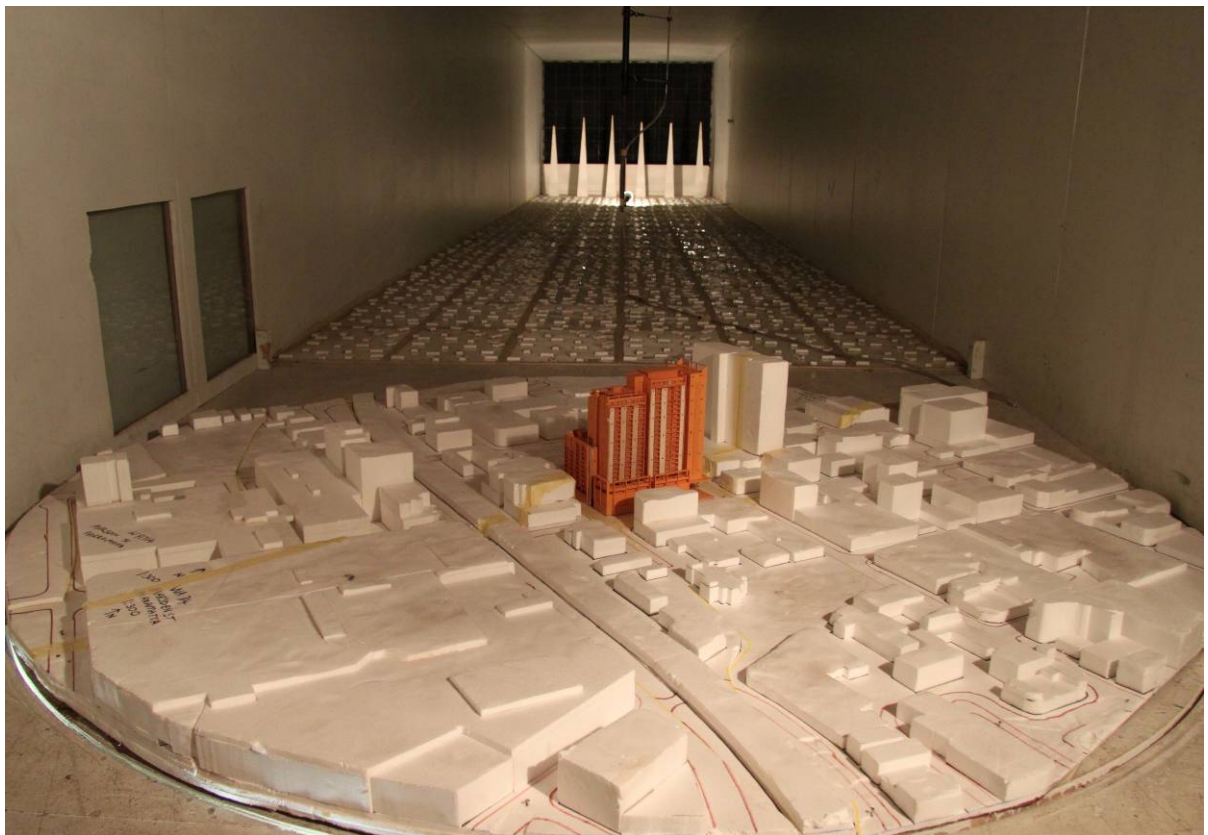
Figure 4a: Photograph of the Model in the Wind Tunnel
