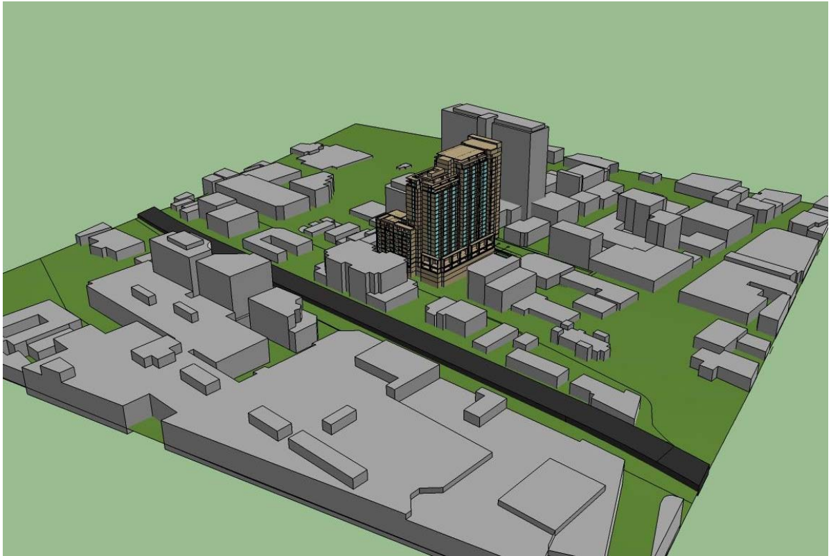
Figure 2b: 3D CAD model used for the Direct Solar Access Study
