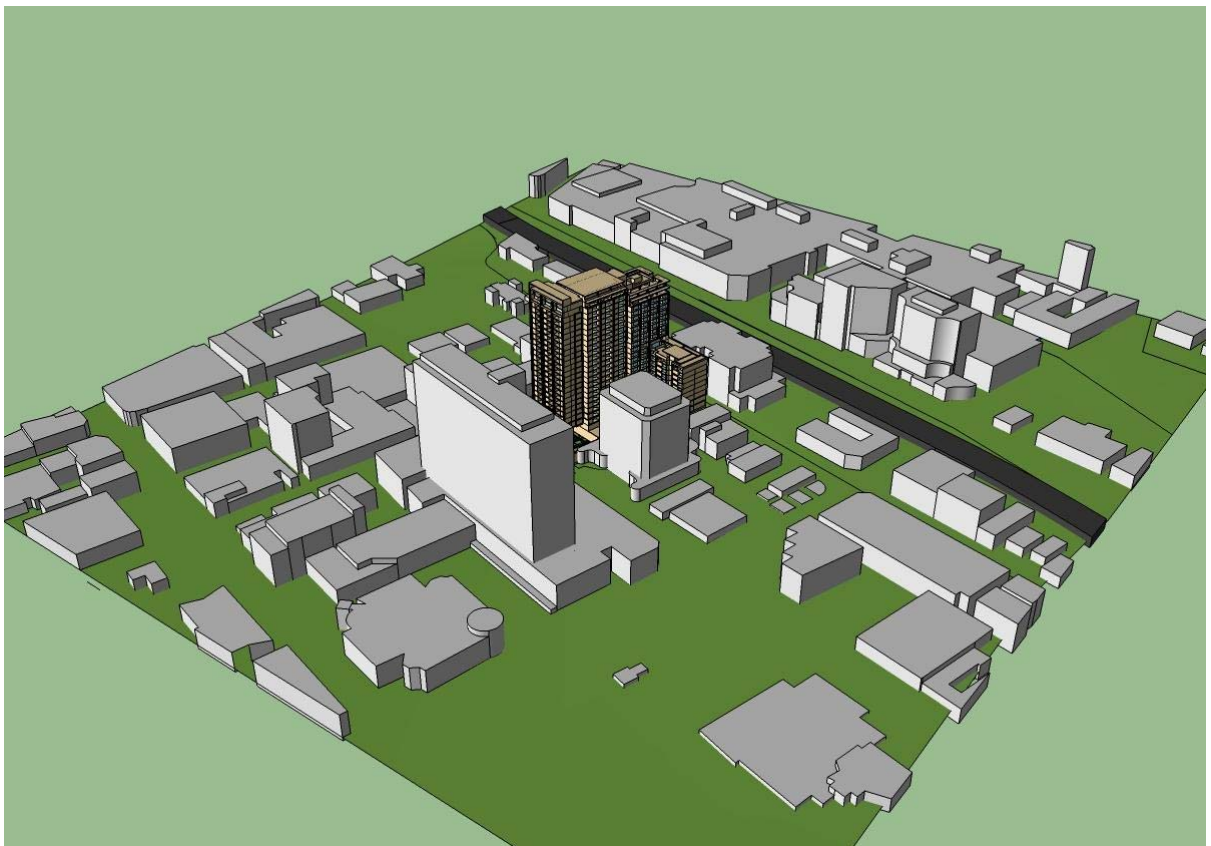
Figure 2c: 3D CAD model used for the Direct Solar Access Study
