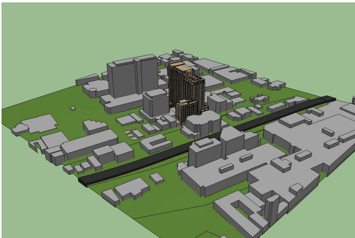
Figure 2d: 3D CAD model used for the Direct Solar Access Study
