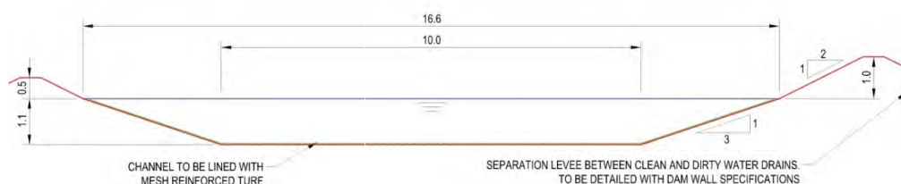
Figure 5-1 Central Clean Water Diversion - Typical Cross Section
