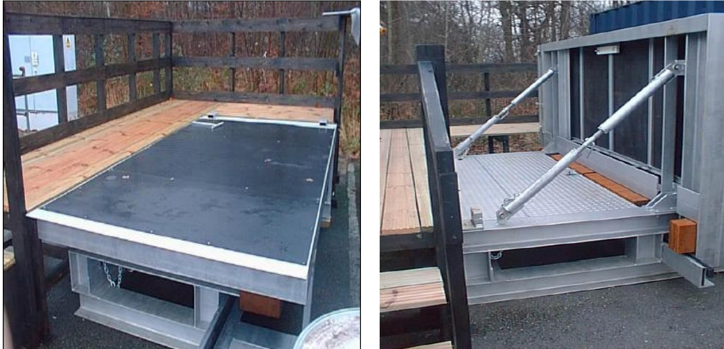
Figure 6.3 Tilt Dam in the closed and opened positions.
