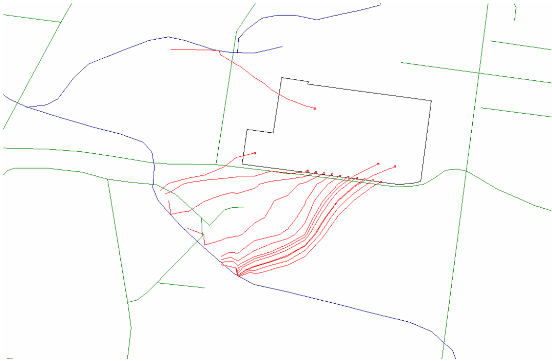
Figure 5.2.5-6. Recharge scenario 2, model layer 3 particle traces.
