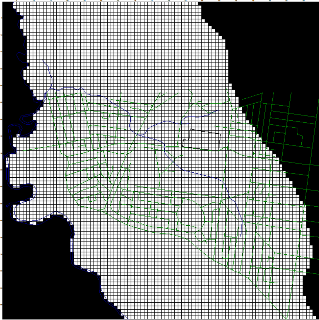
Figure 4.1-1. Model horizontal discretization.
