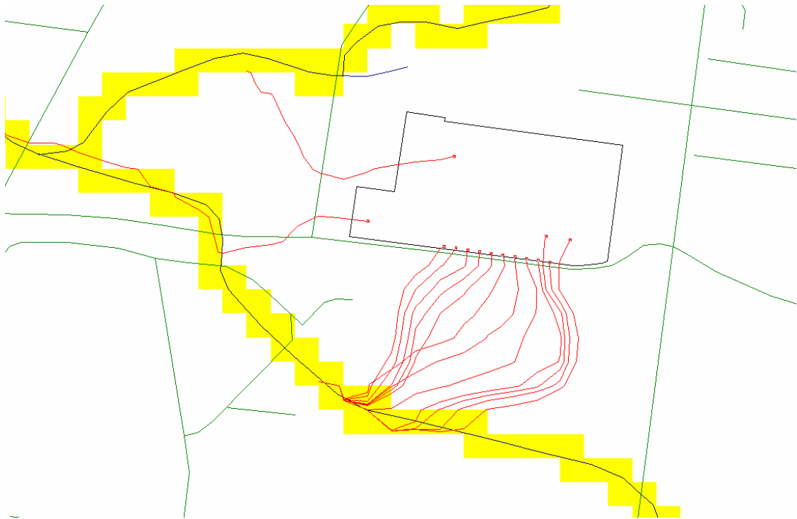
Figure 5.2.5-4. Recharge scenario 2, model layer 1 particle traces.
