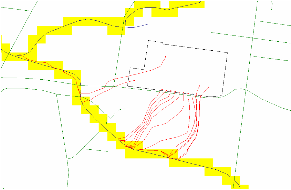
Figure 5.2.5-7. Recharge scenario 3, model layer 1 particle traces.
