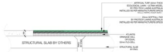
1 ARTIFICIAL TURF ON SLAB TYPICAL SECTION 1:10
