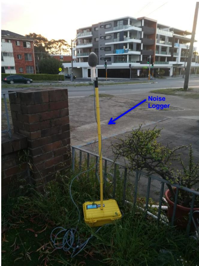
Figure 3 Logger Deployment (234 Gardeners Road)
