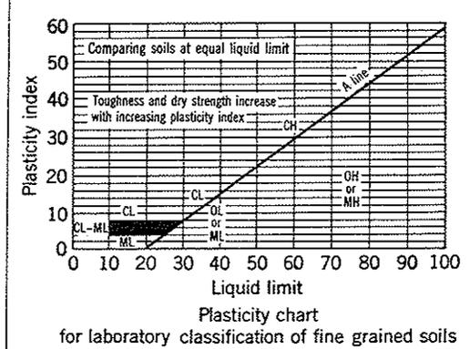
NOTE: 1) Soils possessing characteristics of two groups are designated by combinations of group symbols (e.g. *GW-GC*, well graded gravel-sand mixture with clay fines).
