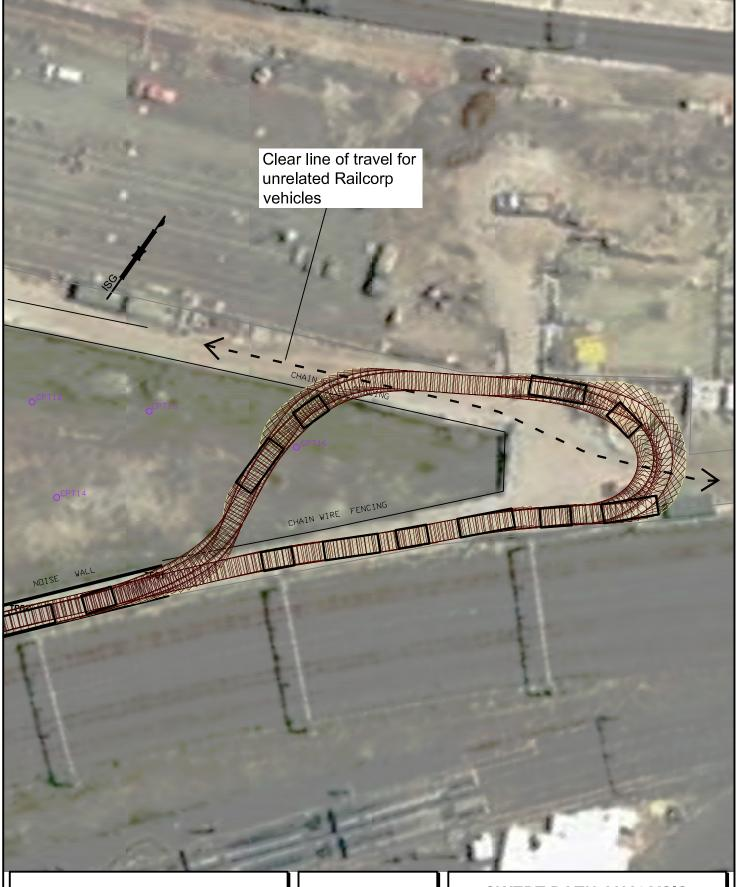
This drawing has been prepared using vehicle modelling computer software AutoTrack V8 in conjunction with AutoCAD 2000. The vehicle used is based upon vehicle data provided by Austroads and incorporates a reasonable degree of tolerance. However, it is not possible to account for all vehicle types/characteristics and/or driver ability.
