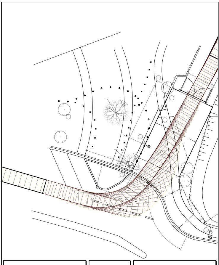
This drawing has been prepared using vehicle modelling computer software AutoTrack V5.00a in conjunction with AutoCAD 2000. The vehicle used is based upon vehicle data provided by Austroads and incorporates a reasonable degree of tolerance. However, it is not possible to account for all vehicle types/characteristics and/or driver ability.
