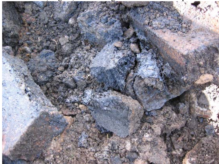
Photo 76 (Aug 06) – Brickwork and tars beneath the former retort house in testpit TP15
