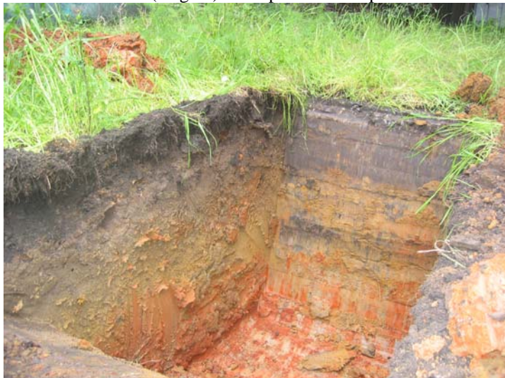
Photo 75 (Aug 06) – Fill profile at testpit TP14, in north western site area
