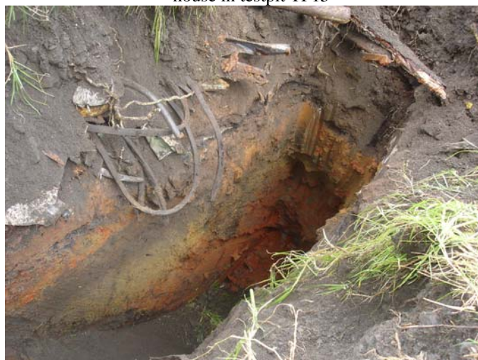
Photo 78 (Aug 06) – Fill profile including waste materials in testpit TP18 (on embankment between gasworks and stabling yard)
