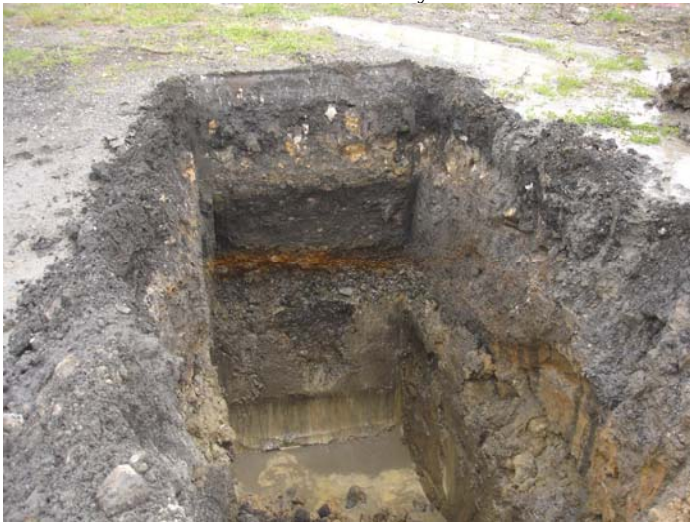
Photo 69 (Aug 06) – Fill profile in testpit TP06, in eastern site area
