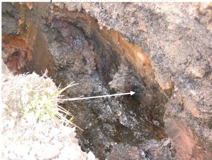
Photo 63 (Aug 06) – Tarry materials and a buried brick structure within testpit MG10, beneath eastern edge of former retort house
