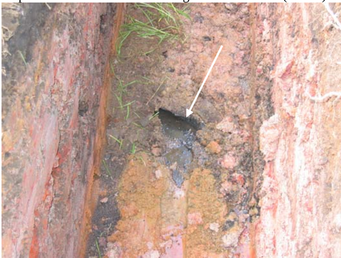
Photo 39 (Aug 06) – Tar pipe and fill layers in testpit MG02, between the two gasholder annuli
