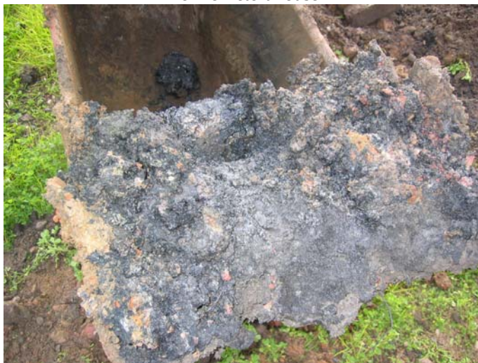
Photo 60 (Aug 06) – Tarry soils within testpit MG08, beneath the former retort house
