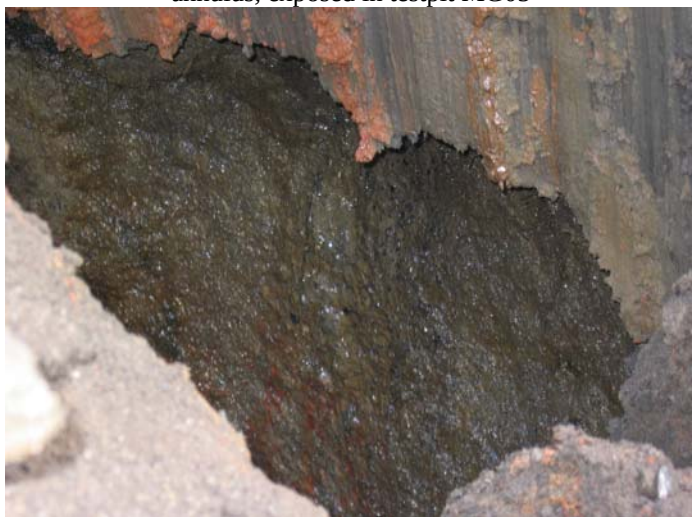
Photo 45 (Aug 06) – Tar and oil seeping into testpit MG05, outside the northern gasholder
