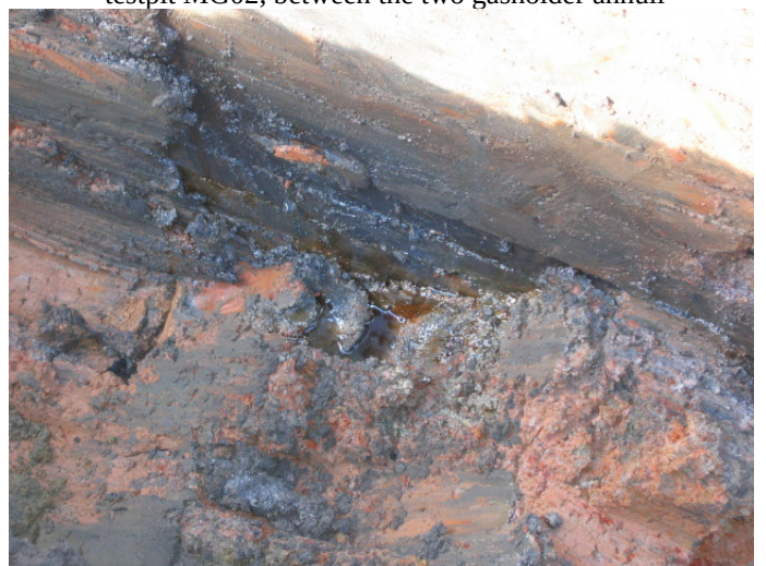
Photo 42 (Aug 06) – Tarry / oily wastes on brickwork – outside of northern gasholder annulus (MG05)
