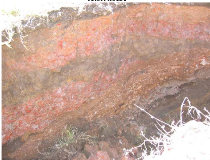
Photo 65 (Aug 06) – Fill layers in testpit MG01, south of existing gasholder
