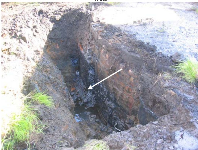
Photo 53 (Aug 06) – Tar seeping through the brick wall of the tar pit (into testpit MG06)
