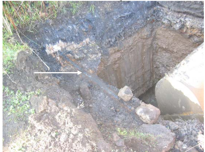
Photo 70 (Aug 06) – Fill profile in testpit TP07, in south eastern site area, including an old buried rail line
