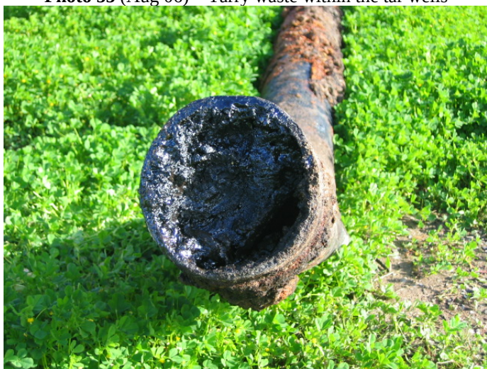
Photo 57 (Aug 06) – Tar within pipework removed from testpit beneath former retort house
