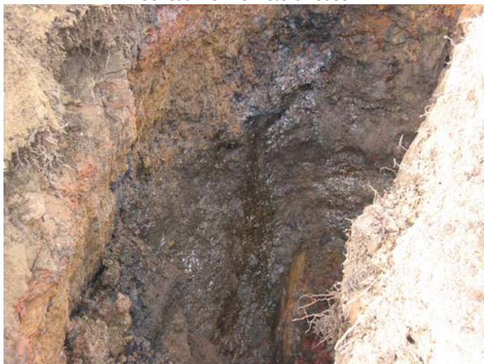
Photo 59 (Aug 06) – Tar within testpit MG08, beneath the former retort house
