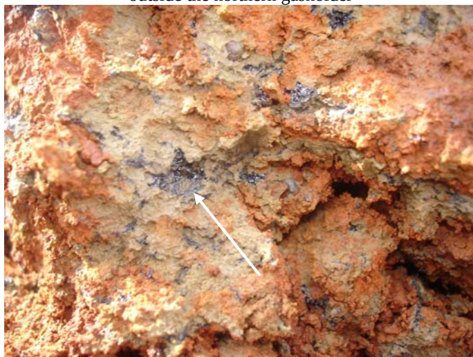
Photo 46 (Aug 06) – Tar within soils pores in natural clay (exact location not documented)
