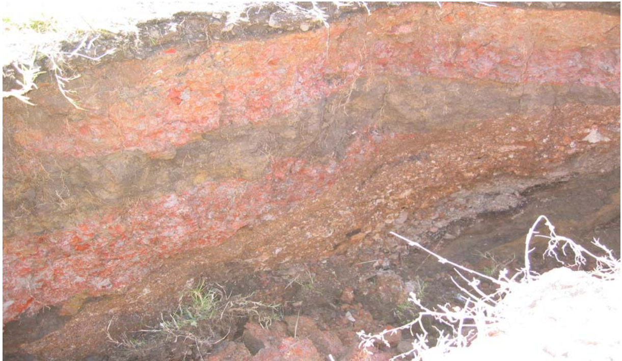
Photo 19 Subsurface conditions showing stratified fill materials at sample location MG01. Indicative material of Gravel, Sand and Clay with Minor Ash across Southwest Area.
