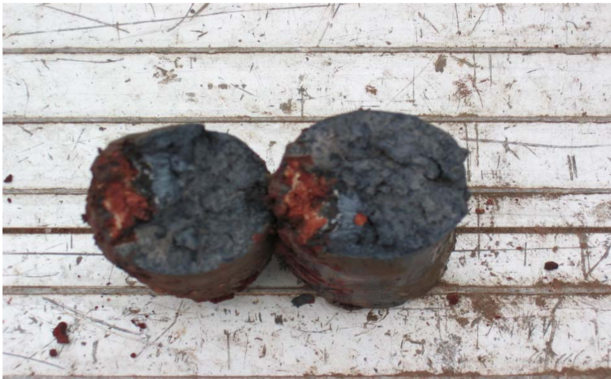
Photo 24 Subsurface conditions showing dark staining in deep weathered shale fractures at sample location BHA at 7.0mbgl.
