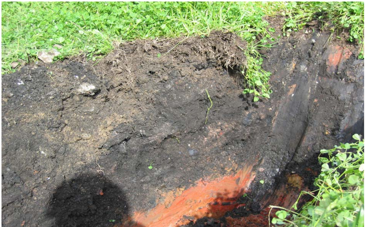
Photo 18 Subsurface conditions showing ash and coke surface fill layer. Profile at sample location MG10.
