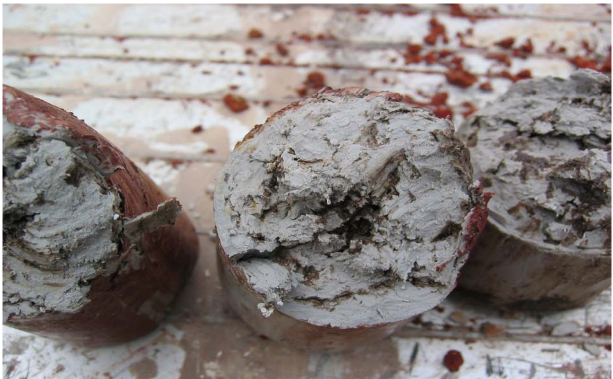
Photo 22 Soil core sample showing free tar in natural soil at sample location BHF at 6.2mbgl.
