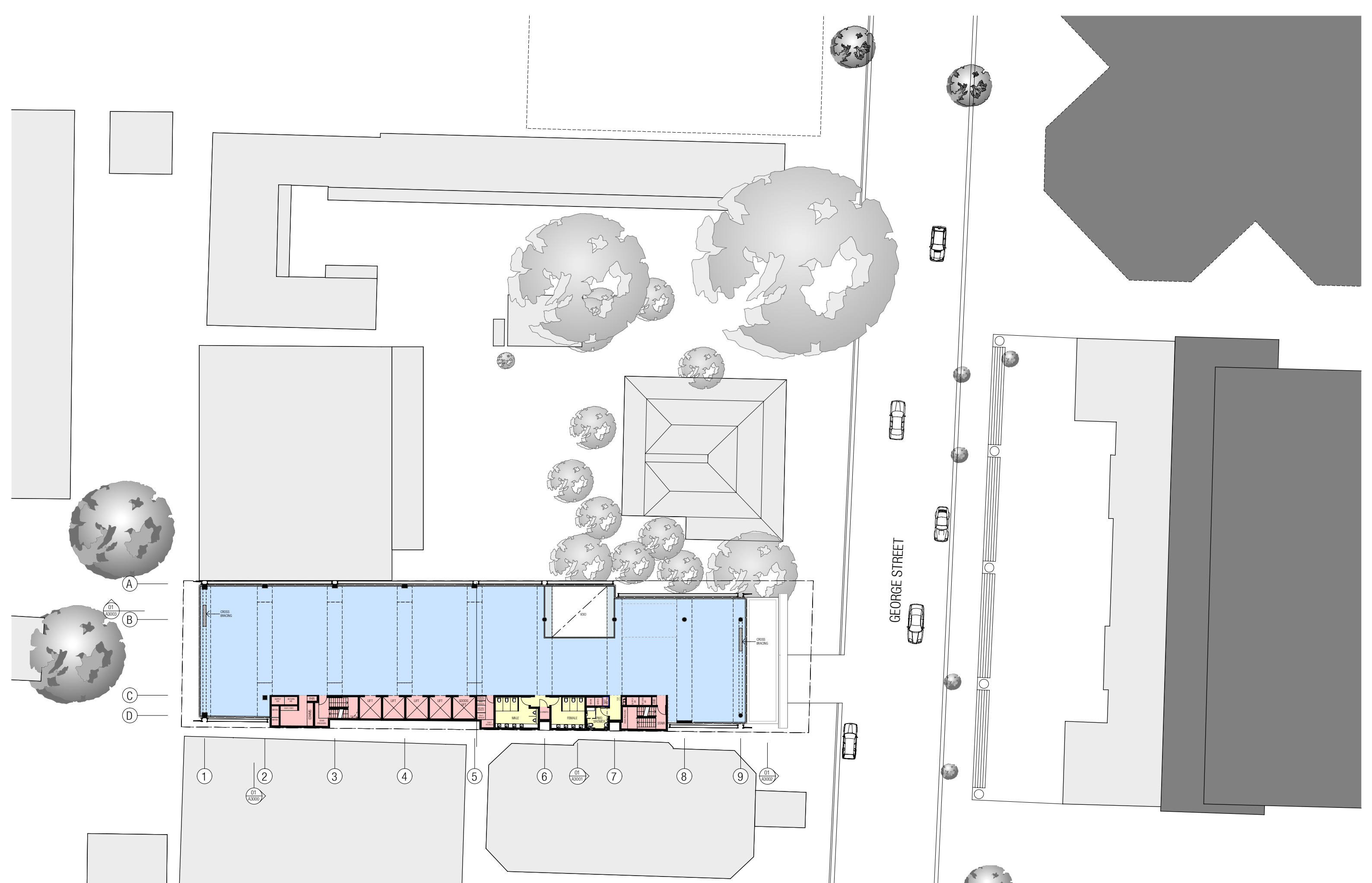
DUXTON DEVELOPMENTS 89 GEORGE STREET FLOOR PLAN - LEVEL 8 - (LEVELS 6-13 TYPICAL)
