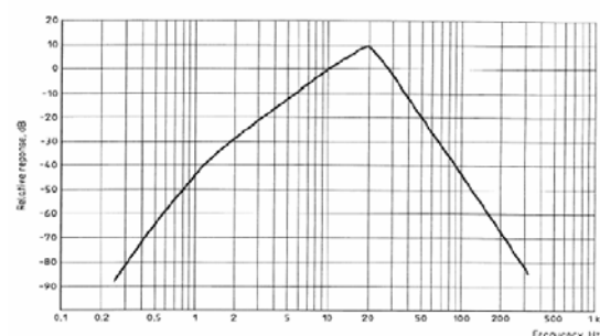
Figure 1: Sound Level Meter Weighting Curves A and C; Figure 2: G-Weighting for Infrasound
