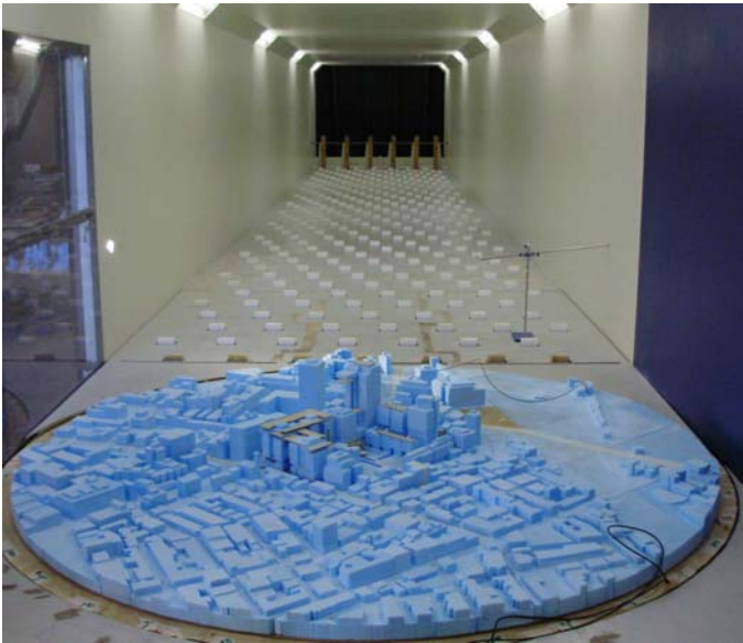
Figure 3: Photograph of Configuration A model in the CPP wind tunnel
