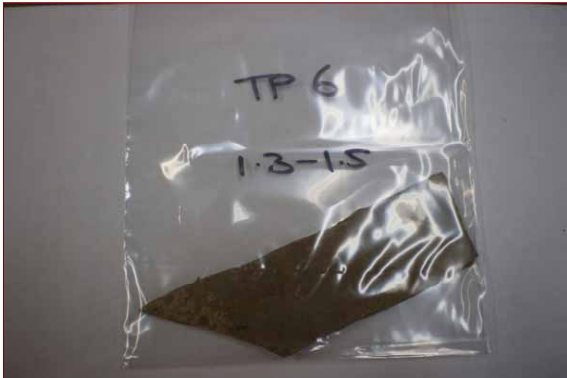
PHOTO 9: A fibre-cement fragment found in TP6 between 1.3 and 1.5 m. Dimension: 90 x 40 mm
