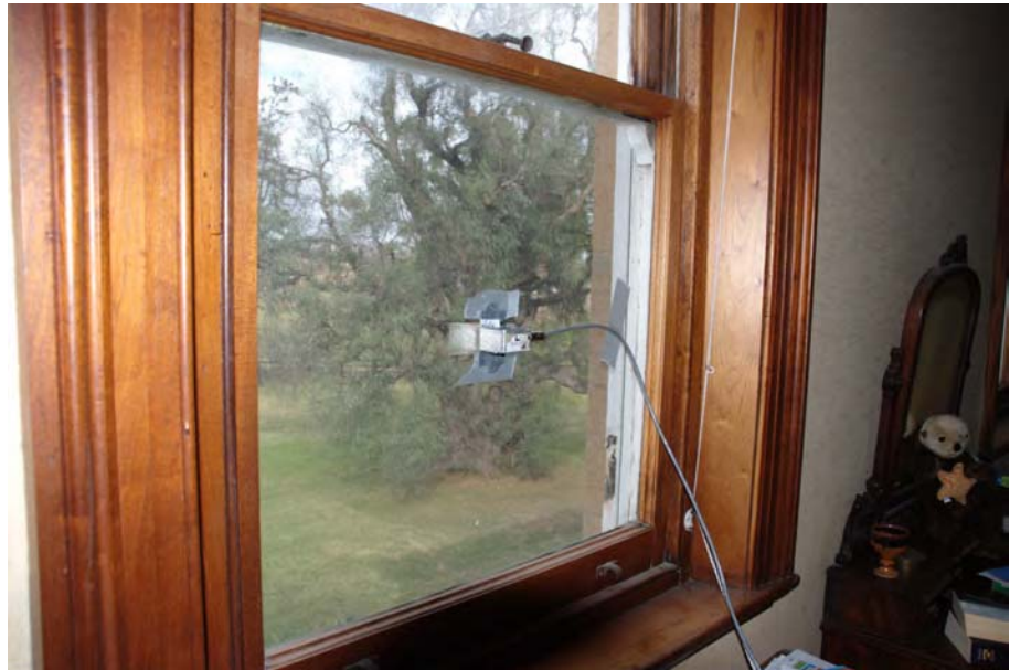
Figure 6: A horizontally oriented sensor was attached to the middle of a typical window pane facing the blast site.
