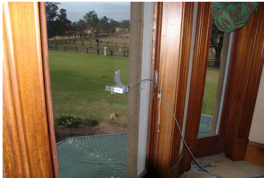
Figure 7: The second horizontal sensor was attached to the lower pane of a french window facing eastwards.
