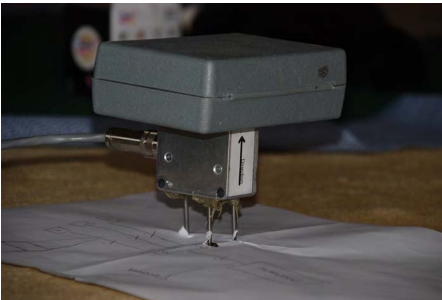
Figure 5: A vertical sensor was set up in the middle of the floor above the games room, rigidly connected to the timber flooring with large nails (the tool box was placed to help secure it).
