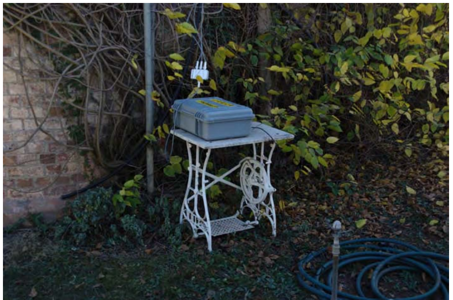
Figure 4: The recorder at the base of the tank stand had a wireless Internet link to the Datamasters headquarters.
