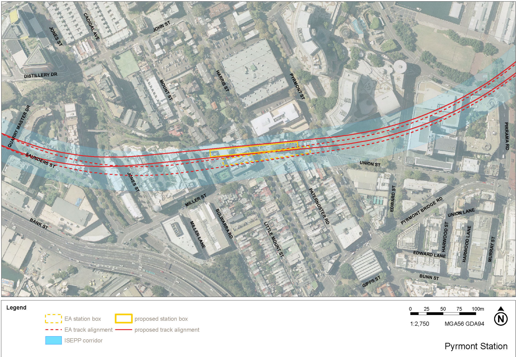
Figure 5.4 Change in project alignment at Pyrmont Station
