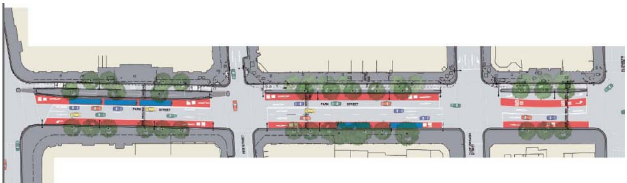
Figure 2.4: Proposed Concept Cycle Lane in Park Street near Town Hall Metro Station
