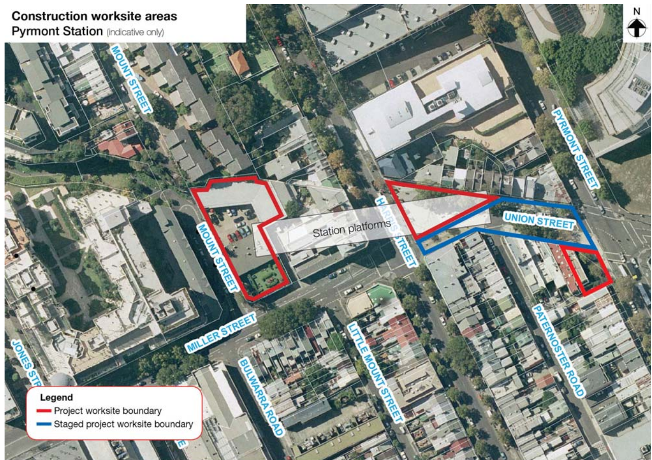
Figure 2.3 Pymont Station construction footprint (indicative only)
