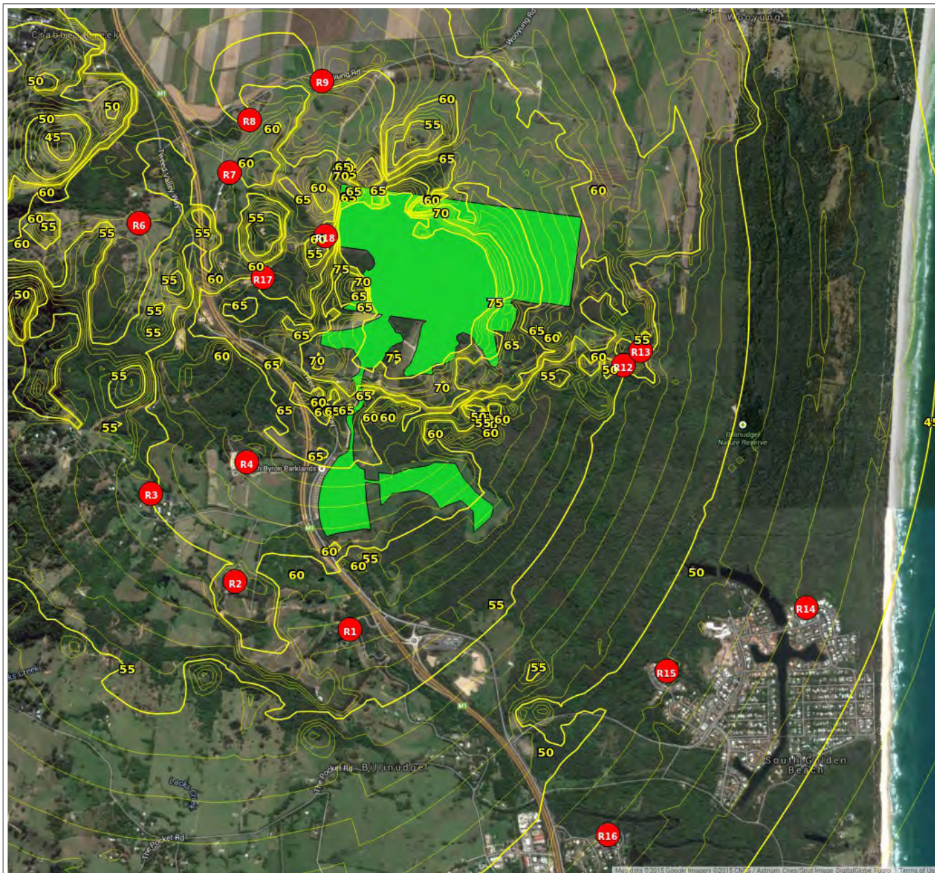
Figure 4.2: Predicted L_{Aeq} Receptor Noise Level Contours - All Stages, Bars, Cafes and Dance-floors (11am-12am)
