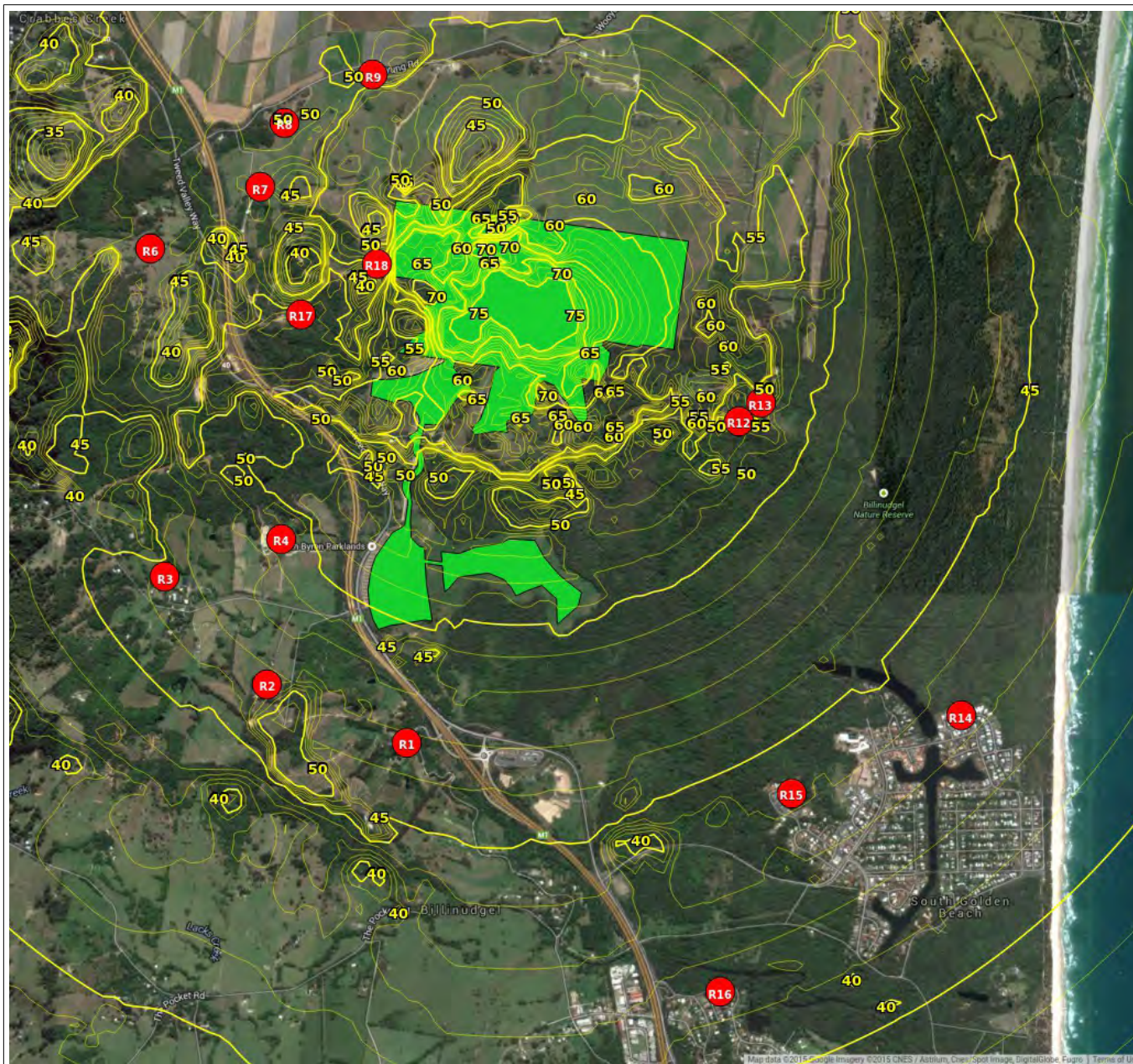
Figure 4.3: Predicted L_{Aeq} Receptor Noise Level Contours – Bars, Cafes and Dance-floors Only (12am-2am)
