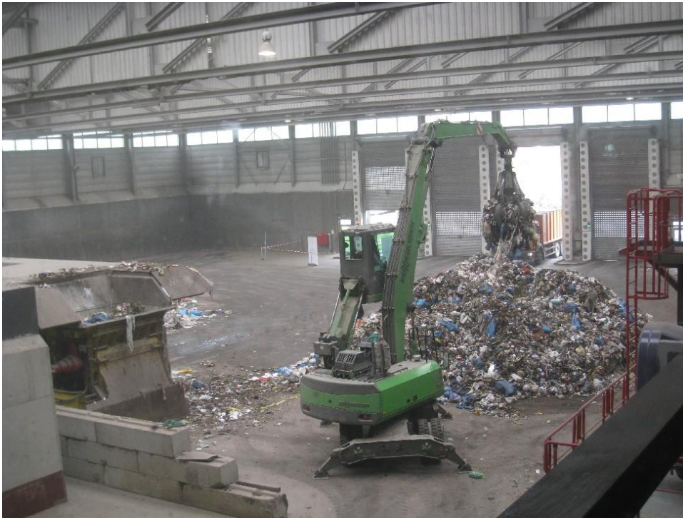
Photo B.2-6 Specialised equipment for removing bulky objects from waste (example)
