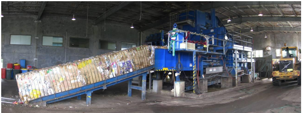
Photo B.2-9 Baling plant at Ballina NSW being used to bale recyclables
