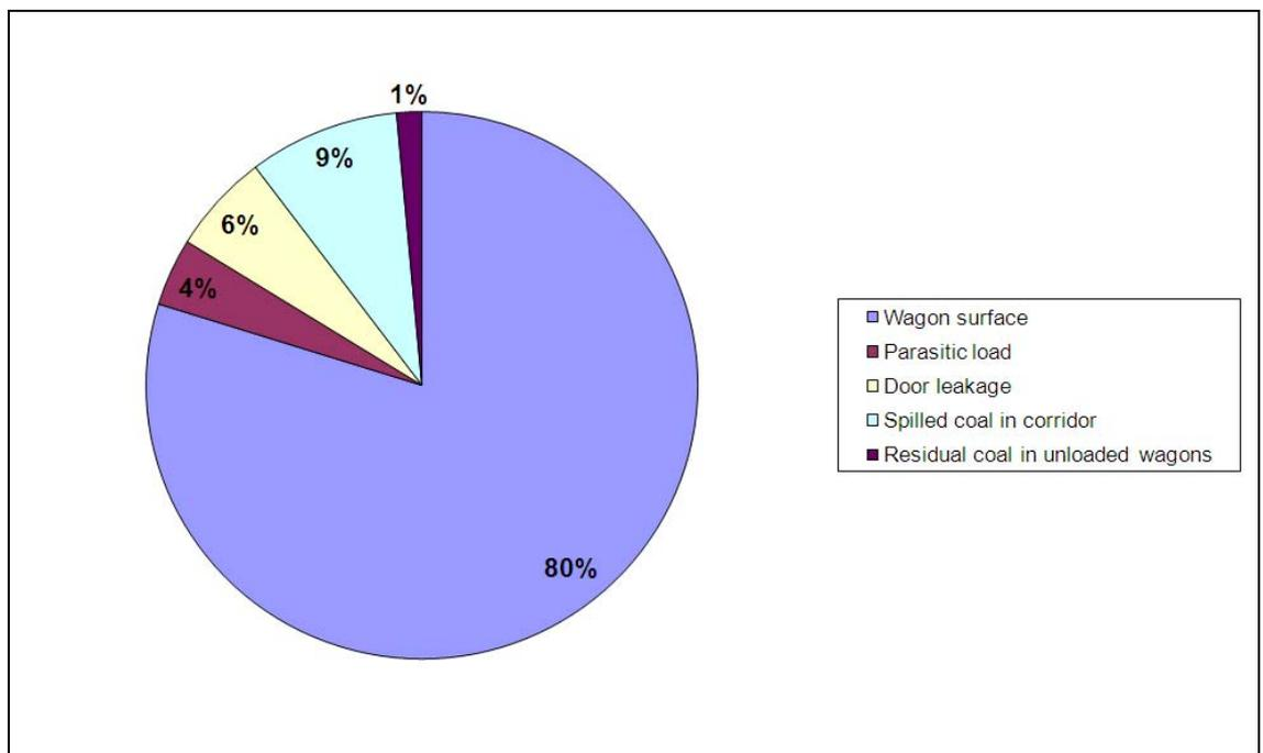
**Figure 6.1 Pie chart showing proportion of coal dust emitted from the wagon surface, door leakage, spilled coal in the corridor, parasitic load and residual coal in unloaded wagons**
