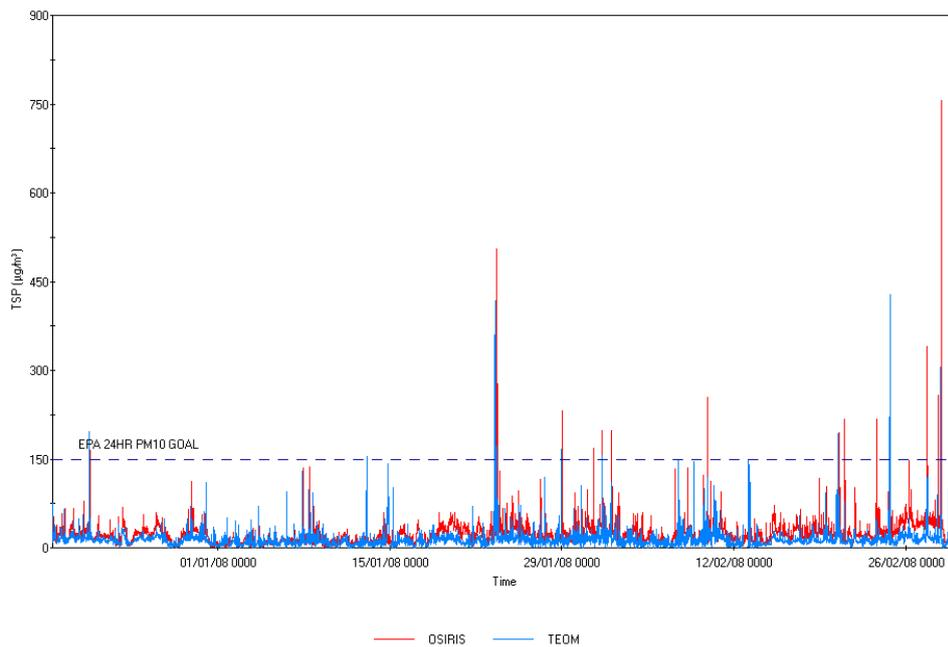
Figure 34. 10 minute average concentration of TSP ( $\mu\text{g}/\text{m}^3$ ) measured at 10 metres from the tracks at Earlsfield for the time period December 18 2007 to February 29 2008. The blue line represents the TEOM and the red line is the Osiris
