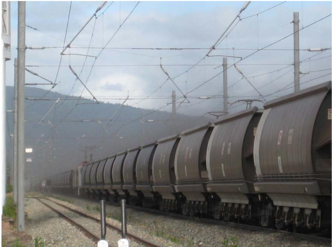
**Figure 4.1** Photograph showing an example of coal dust emitted from the surface of coal wagons (Photograph taken by Jim Harrison on 15 December 2007 at Nebo road turnoff on Goonyella System)
