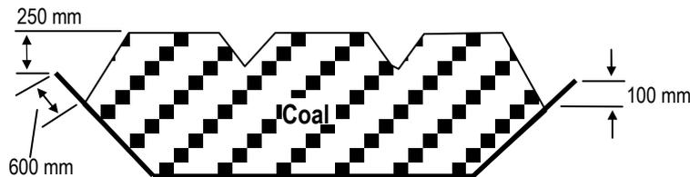
Figure 2 Dimensions of three mound ('clamshell') coal configuration
