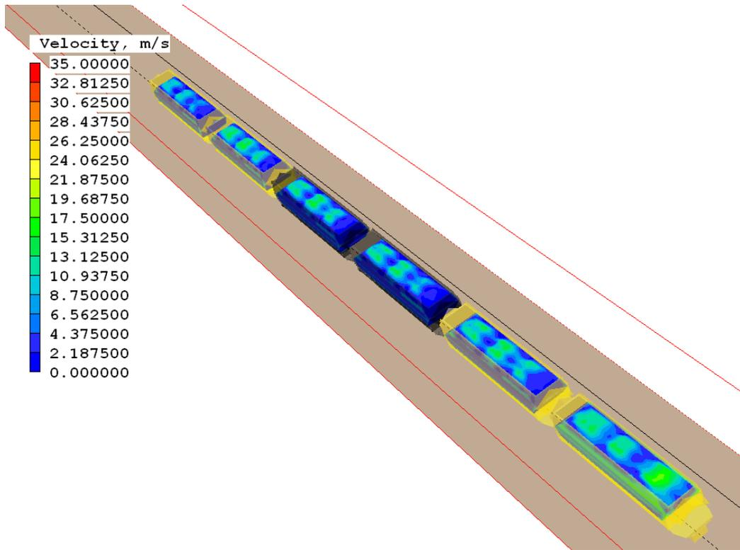
Figure 6.1.1d Model 2 – Unmodified wagon and three mound coal configuration velocity contour coal surface velocity
