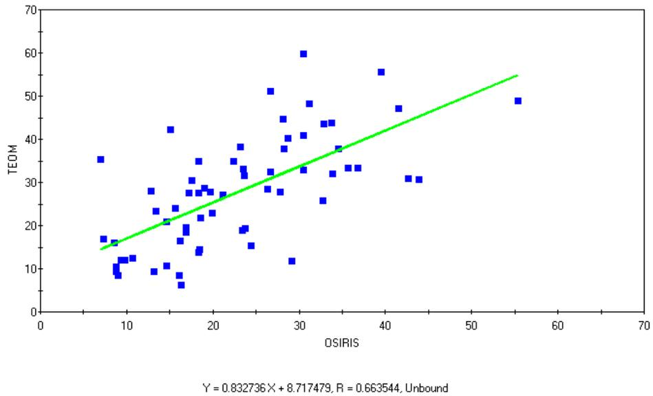
Figure 33. Regression analysis of TEOM versus Osiris 24 hour average TSP ( $\mu\text{g}/\text{m}^3$ ) with an R value of 0.66 for Boonal during the time period December 31 2007 to March 6 2008
