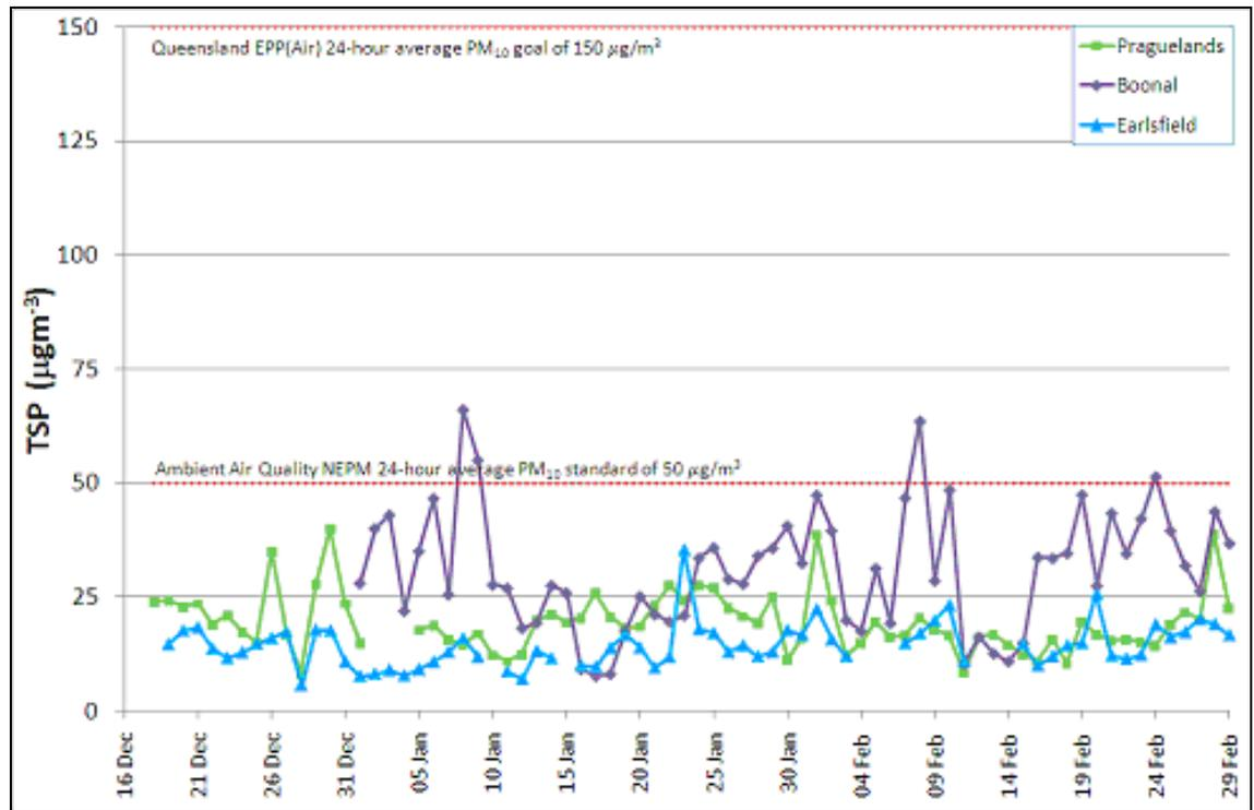
Figure 7.7 24-hour average concentration of TSP ( $\mu\text{g}/\text{m}^3$ ) measured at about 10 metres from the tracks at Praguelds, Boonal and Earlsfield (December 2007 to 29 February 2008)
