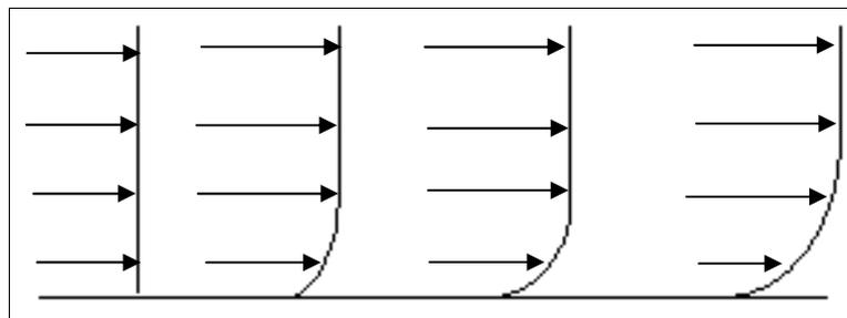
Figure 10 Generation of Wind Profile in Wind Tunnel
