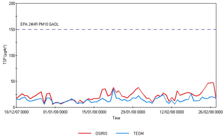
Figure 37. 24 hour average Concentration of TSP ( $\mu\text{g}/\text{m}^3$ ) measured at 10 metres from the tracks at Earlsfield for the time period December 18 2007 to February 29 2008. The blue line represents the TEOM and the red line is the Osiris
