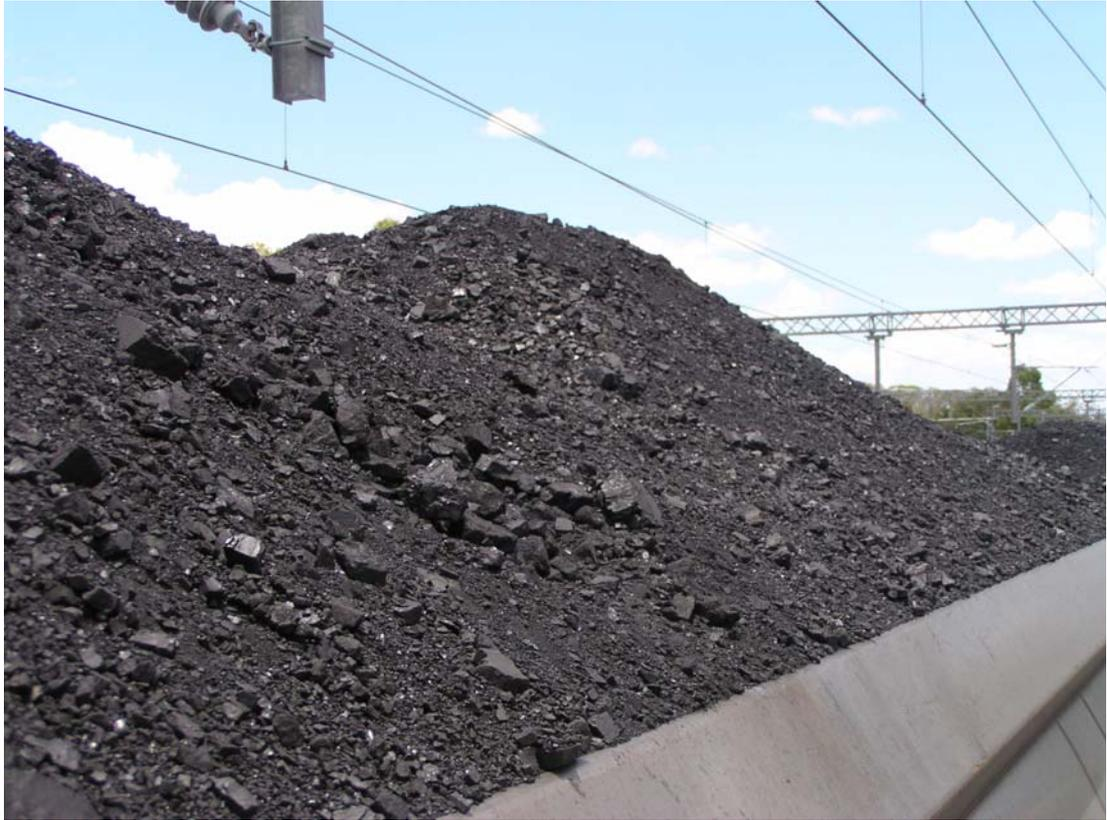
**Figure 5.3** Photograph showing a poorly loaded wagon
