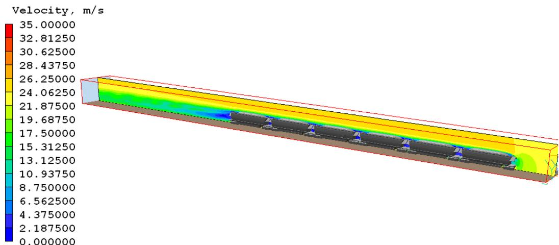
Figure 6.1.1a Model 1 – Unmodified wagon and single mound coal configuration velocity contour isometric
