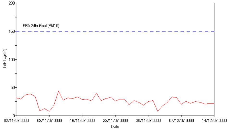
Figure 4. 24 hour average Mass Concentration of TSP ( $\mu\text{g}/\text{m}^3$ ) measured at 10 metres from the tracks at Beecher (November 11 to December 13 2007)
