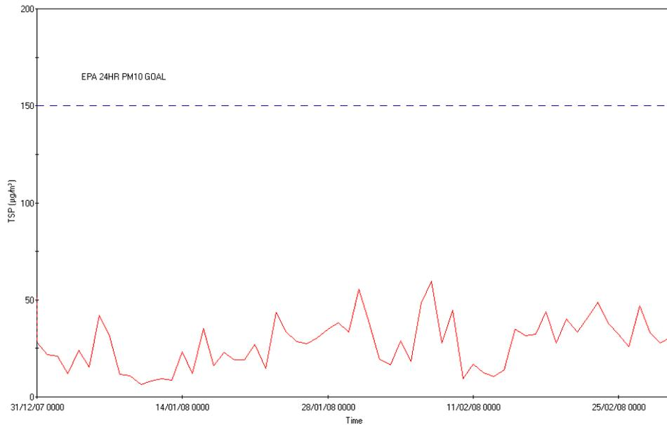
Figure 17. 24 hour average Concentration of TSP ( $\mu\text{g}/\text{m}^3$ ) measured at 10 metres from the tracks at Boonal (December 31 2007 to March 06 2008)
