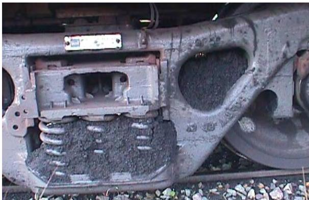
Figure 5 - Parasitic Load in Spring Nests
