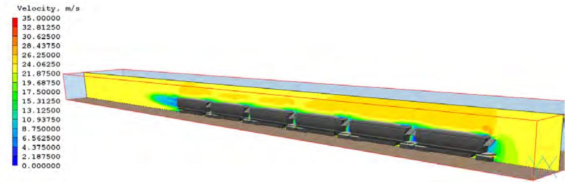
Figure 6.1.2e Model 3 – Wagon with 300 mm hungry board and single mound coal configuration velocity contour isometric
