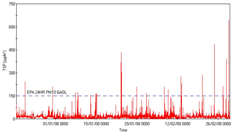
Figure 7. 5-minute average Mass Concentration of TSP ( $\mu\text{g}/\text{m}^3$ ) measured at 10 metres from the tracks at Earlsfield (December 18 2007 to February 29 2008)
