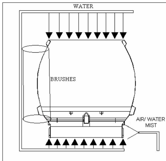
Figure 10 – Air / Water / Brush Combination Method
