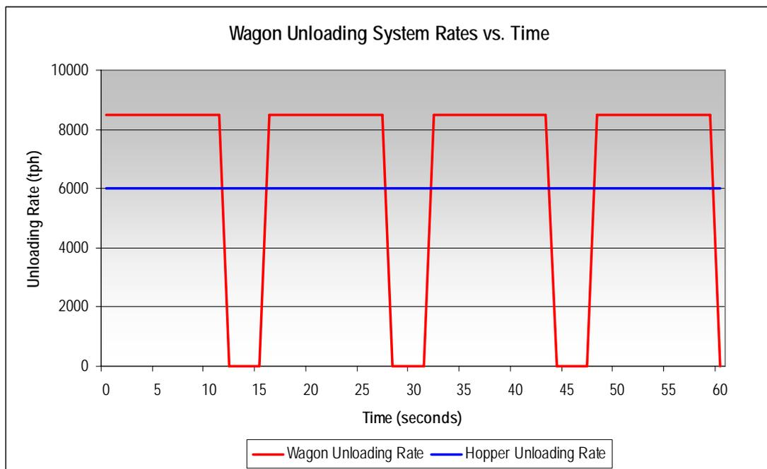
Figure 1 – Indicative Wagon Unloading System Rates vs. Time
