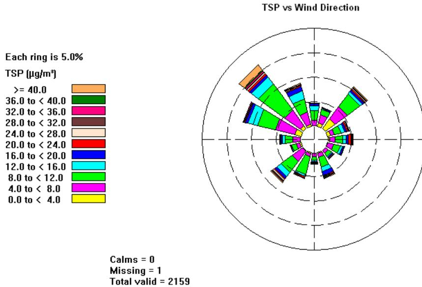
**Figure 28.** Wind/Dust rose of 5-minute average wind speed (m/s) and wind direction measured at 10 metres from the tracks at Mindi (January 14 to February 26 2008). The directional spread of the columns indicates a predominance of North West wind components; the coloured portion of the columns is TSP concentration
