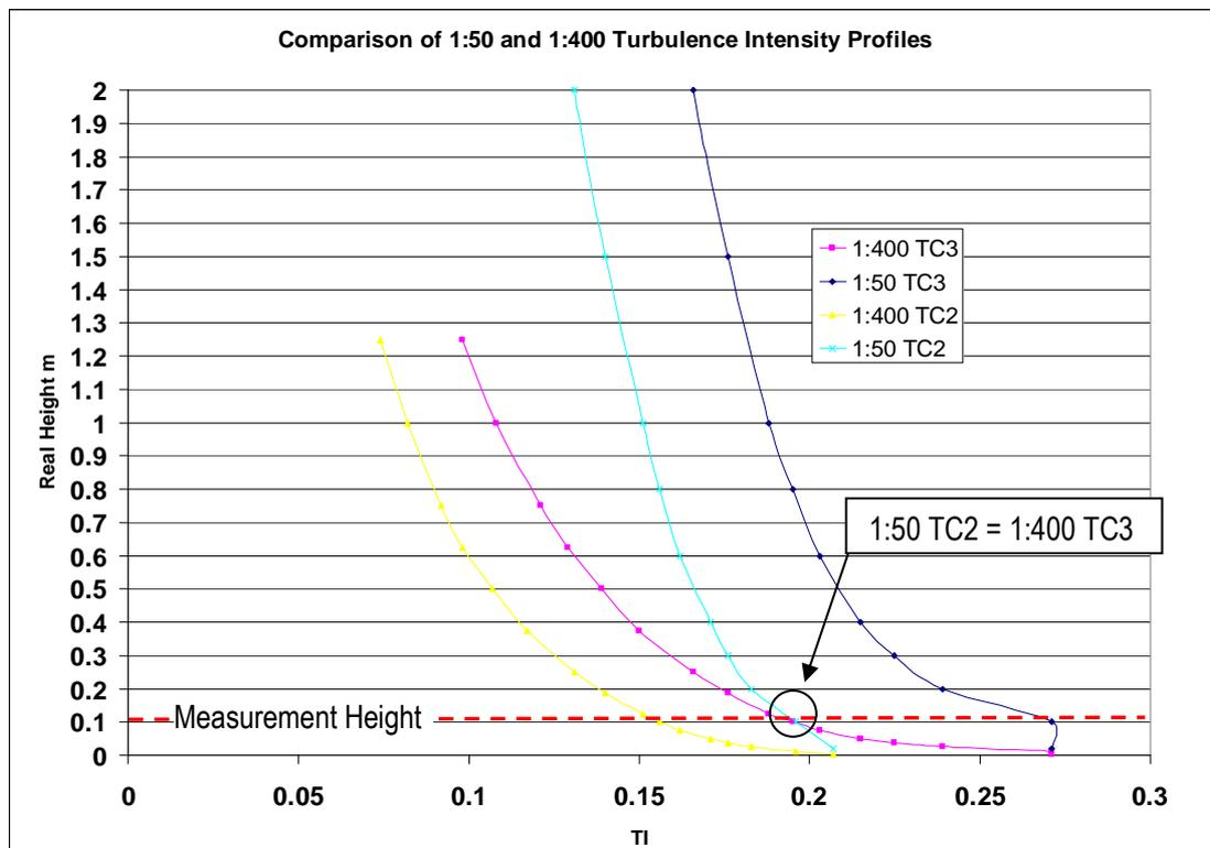
Figure 8 Turbulence Intensity Profiles (Source: AS1170.2)
