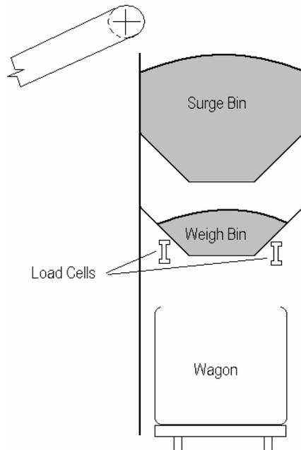
Figure 2 – Batch Weighing System
