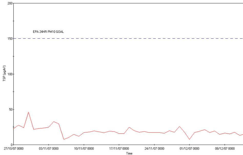
Figure 13. 24 hour average Concentration of TSP ( $\mu\text{g}/\text{m}^3$ ) measured at 10 metres from the tracks at Raglan (October 22 to December 13 2007)
