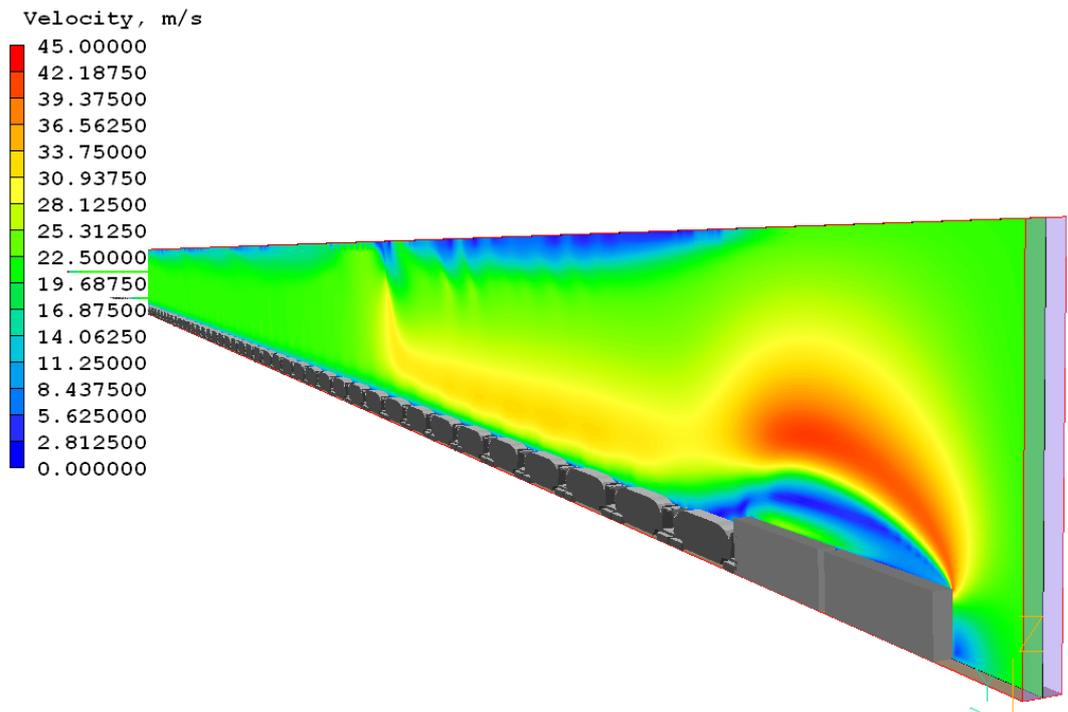
Figure 6.1.1g Model 4 – Unmodified wagon and single mound coal configuration velocity contour isometric with addition of locomotive
