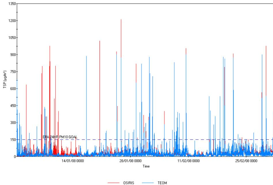
**Figure 29.** 10 minute average concentration of TSP ( $\mu\text{g}/\text{m}^3$ ) measured at 10 metres from the tracks at Boonal for the time period December 31 2007 to March 6 2008. The blue line represents the TEOM and the red line is the Osiris
