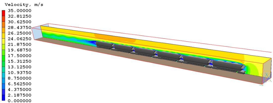
Figure 6.1.1e Model 3 – Wagon with 300 mm hungry board and three mound coal configuration velocity contour isometric
