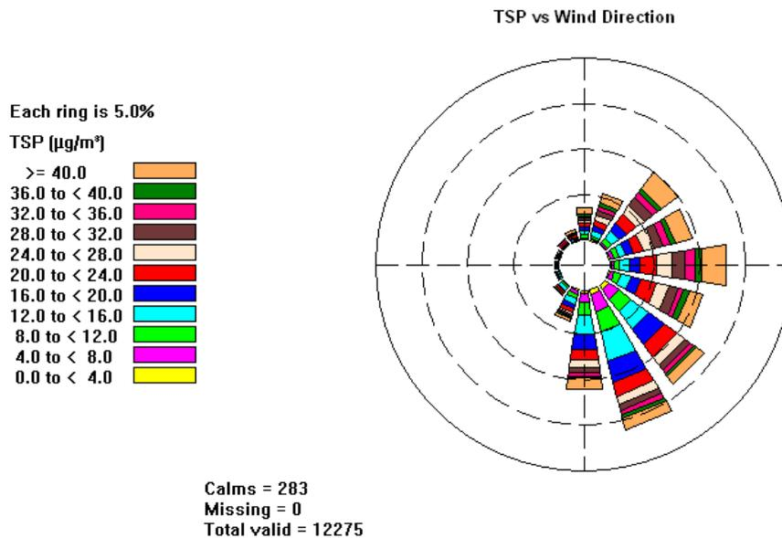
Figure 5. Wind/Dust rose of 5-minute average wind direction and TSP ( $\mu\text{g}/\text{m}^3$ ) measured at 10 metres from the tracks at Beecher (November 11 to December 13 2007). The directional spread of the columns indicates a predominance of East to South East wind components; the coloured portion of the columns is TSP concentration
