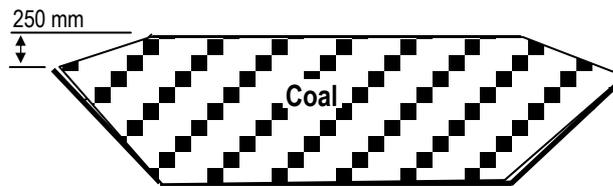
Figure 5 Tee Pee Load
