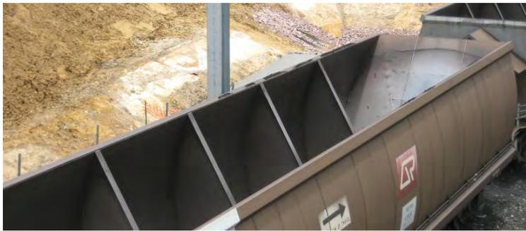
Figure 3 – Parasitic Load on Wagon Sills
