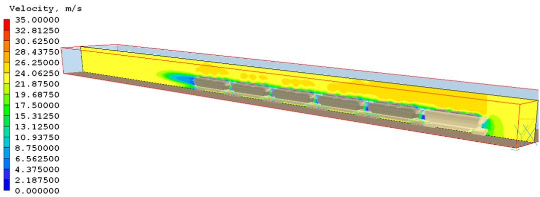
Figure 6.1.2c Model 2 – Unmodified wagon and three mound coal configuration velocity contour isometric
