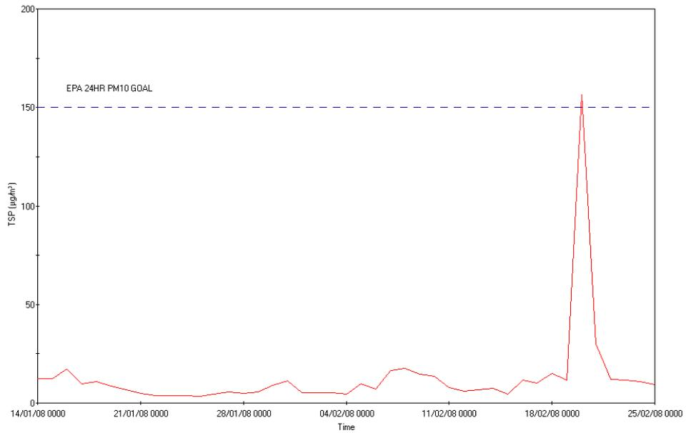
Figure 26. 24 hour average Concentration of TSP ( $\mu\text{g}/\text{m}^3$ ) measured at 10 metres from the tracks at Mindi (January 14 to February 26 2008)
