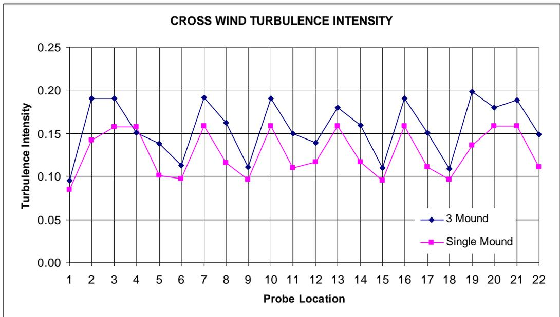
Figure 6.2.2b Turbulence intensity profile – cross wind case
