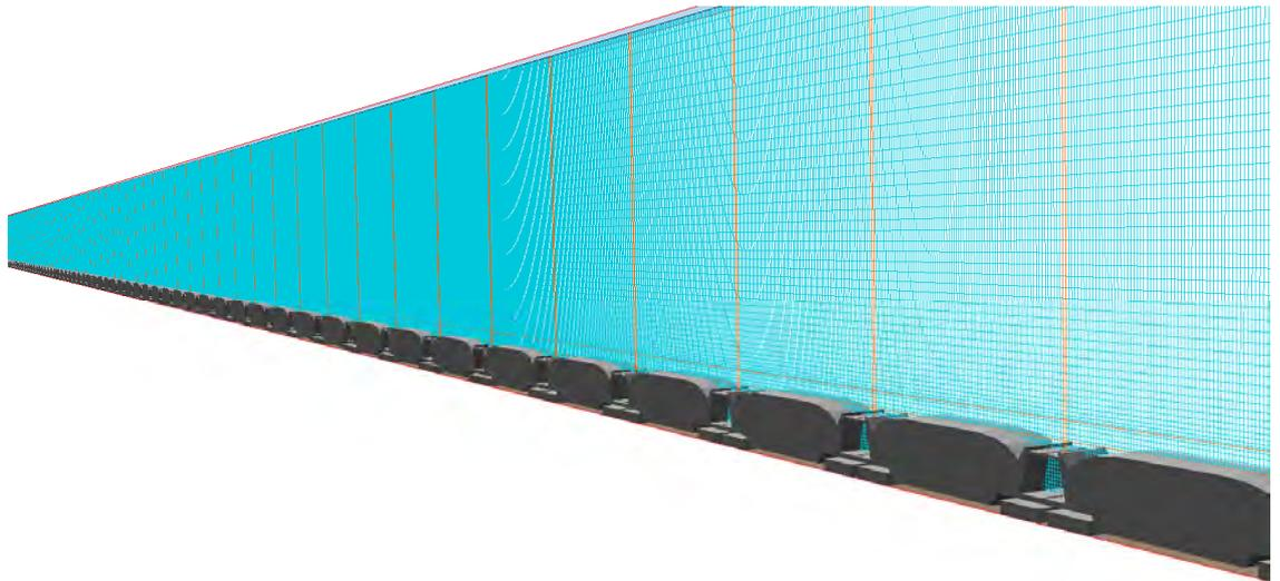
Figure 4 Isometric view of 100 Inline wagons 2D analysis.
