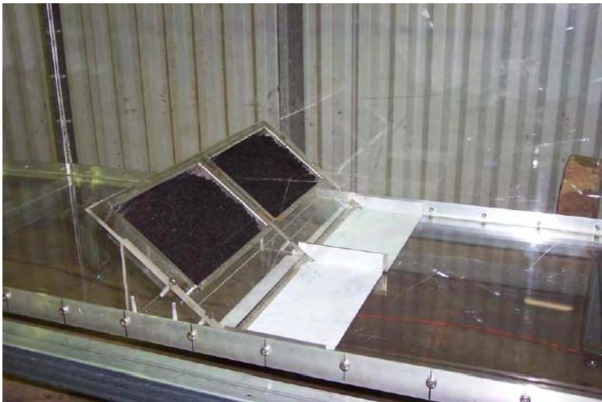
**Figure C 1 Wind tunnel with two sample trays**
