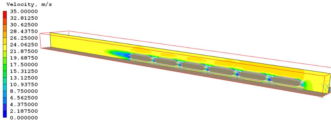
Figure 6.1.2a Model 1 – Unmodified wagon and single mound coal configuration velocity contour isometric
