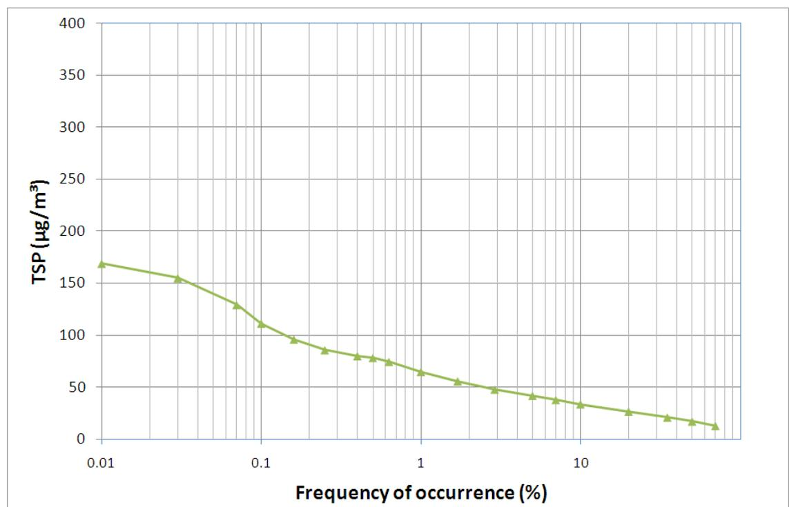
**Figure 7.8 Cumulative frequency distributions of 1-hour average concentrations of TSP ( $\mu\text{g}/\text{m}^3$ ) measured at about 10 metres from the edge of tracks at Callemondah from April to October 2007.**
