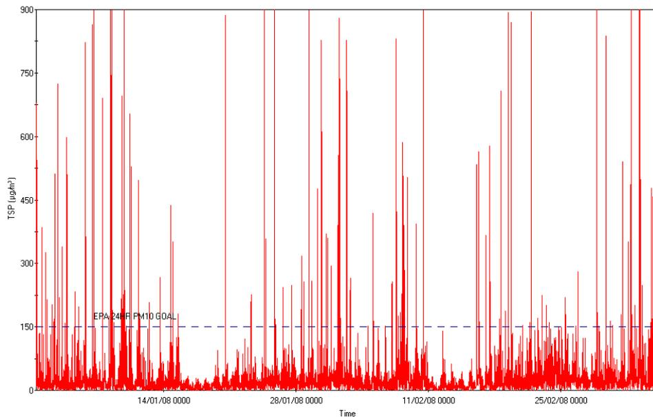
Figure 16. 5-minute average Concentration of TSP ( $\mu\text{g}/\text{m}^3$ ) measured at 10 metres from the tracks at Boonal (December 31 2007 to March 6 2008)
