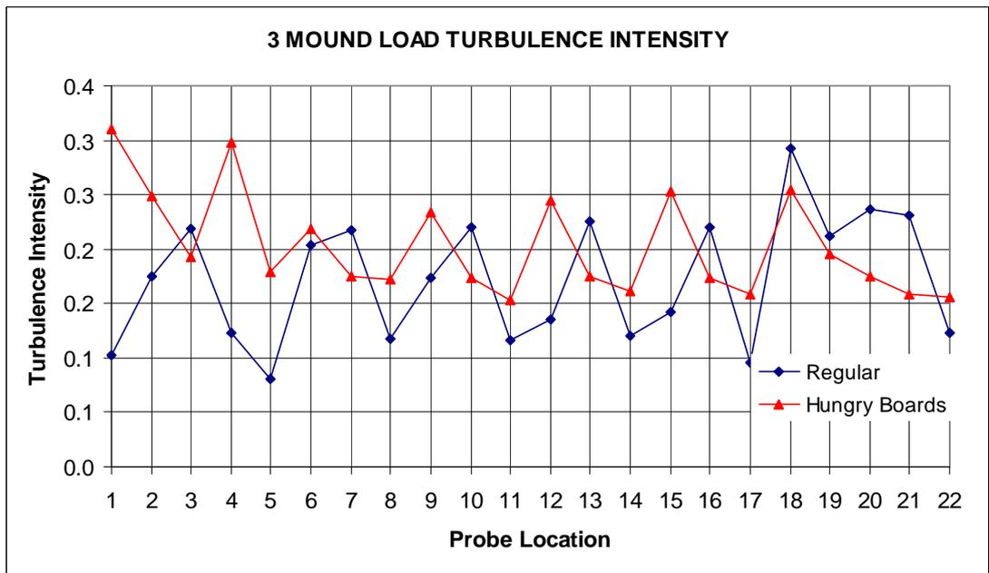
Figure 6.2.1d Turbulence intensity profile – 3 mound case
