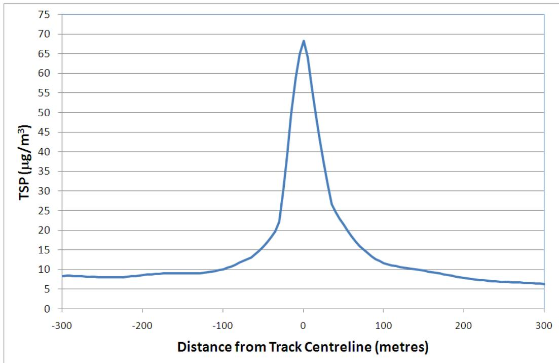
**Figure 7.16 Scenario 2. Cross-section of predicted maximum 24-hour average ground-level concentration of TSP ( $\mu\text{g}/\text{m}^3$ ) due to 2006/07 train movements on the Blackwater System. Train speed is 80 km/hr.**
