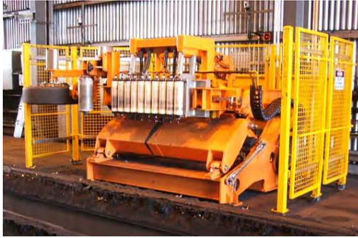
Figure 7 – Automatic Wagon Vibrator
