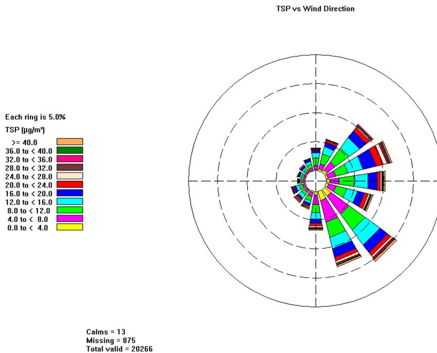
Figure 9. Wind/Dust rose of 5-minute average wind direction and TSP ( $\mu\text{g}/\text{m}^3$ ) measured at 10 metres from the tracks at Earlsfield (December 18 2007 to February 29 2008). The directional spread of the columns indicates a predominance of East to South East wind components; the coloured portion of the columns is TSP concentration
