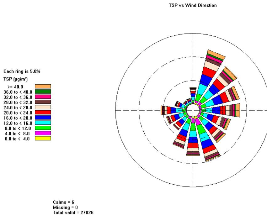
Figure 23. Wind rose of 5-minute average wind speed (m/s) and wind direction measured at 10 metres from the tracks at Praguelds (November 11 2007 to February 29 2008). The directional spread of the columns indicates a predominance of North East and South East wind components; the coloured portion of the columns is TSP concentration
