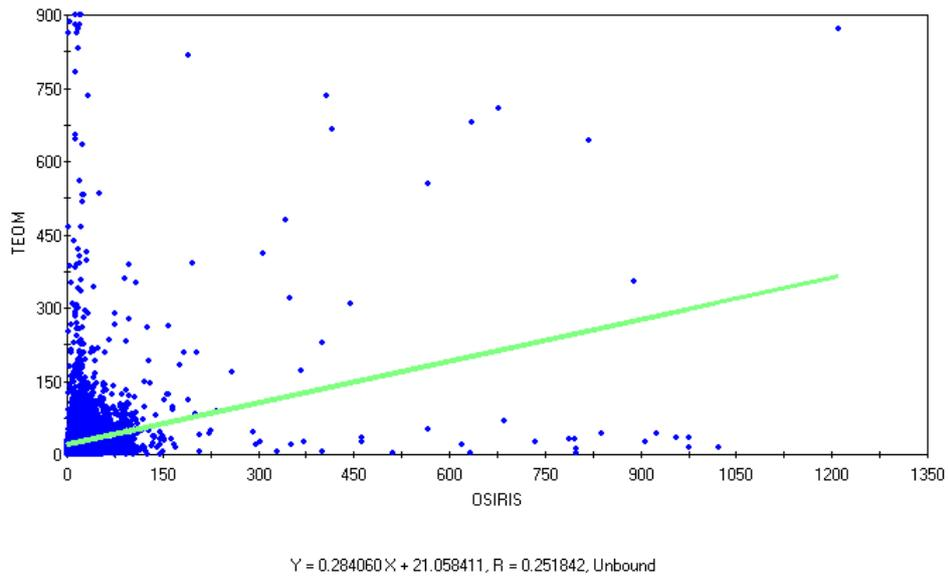
Figure 31. Regression analysis of TEOM versus Osiris 24 hour average TSP ( $\mu\text{g}/\text{m}^3$ ) with an R value of 0.25 for Boonal during the time period December 31 2007 to March 6 2008
