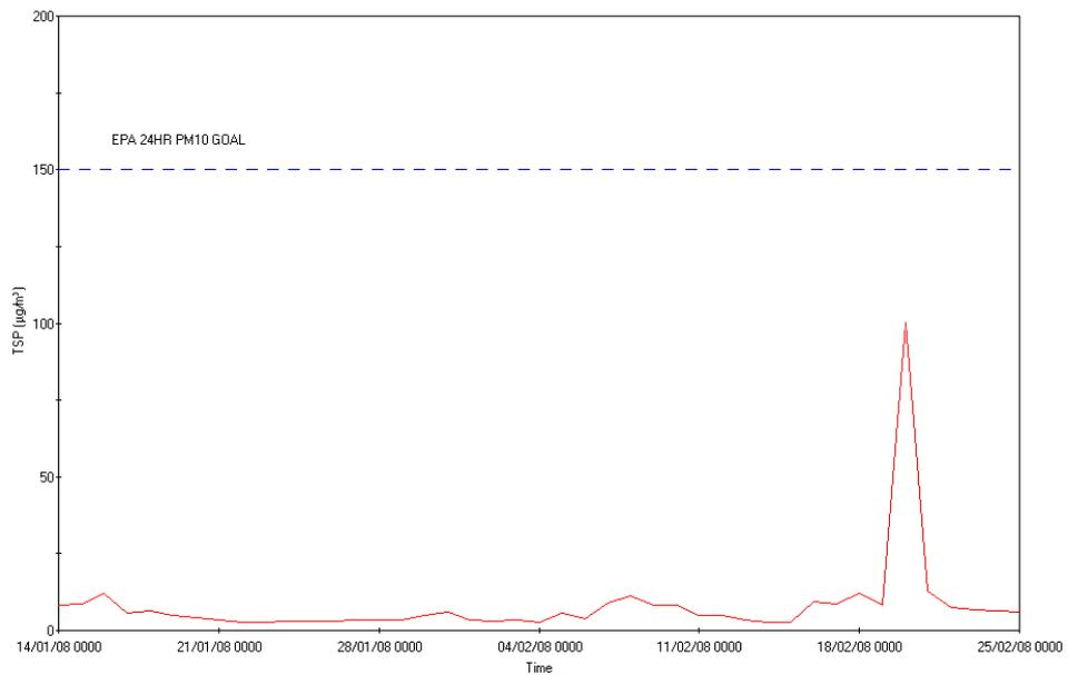
Figure 27. 24 hour average Concentration of PM10 ( $\mu\text{g}/\text{m}^3$ ) measured at 10 metres from the tracks at Mindi (January 14 to February 26 2008)
