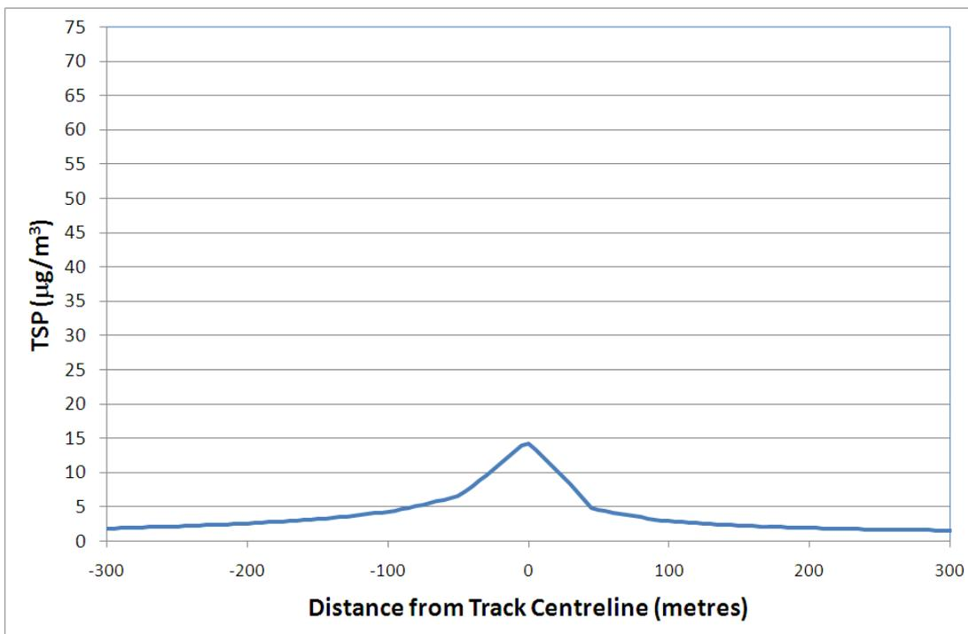
Figure 7.14 Scenario 1. Cross-section of predicted maximum 24-hour average ground level concentration of TSP ( $\mu\text{g}/\text{m}^3$ ) due to 2006/07 train movements on the Goonyella system. Train speed is 38 km/hr.
