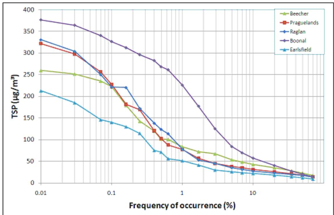
**Figure 7.9 Cumulative frequency distributions of 1-hour average concentrations of TSP ( $\mu\text{g}/\text{m}^3$ ) measured at about 10 metres from the edge of tracks at Beecher, Praguelds, Raglan, Boonal and Earlsfield.**
