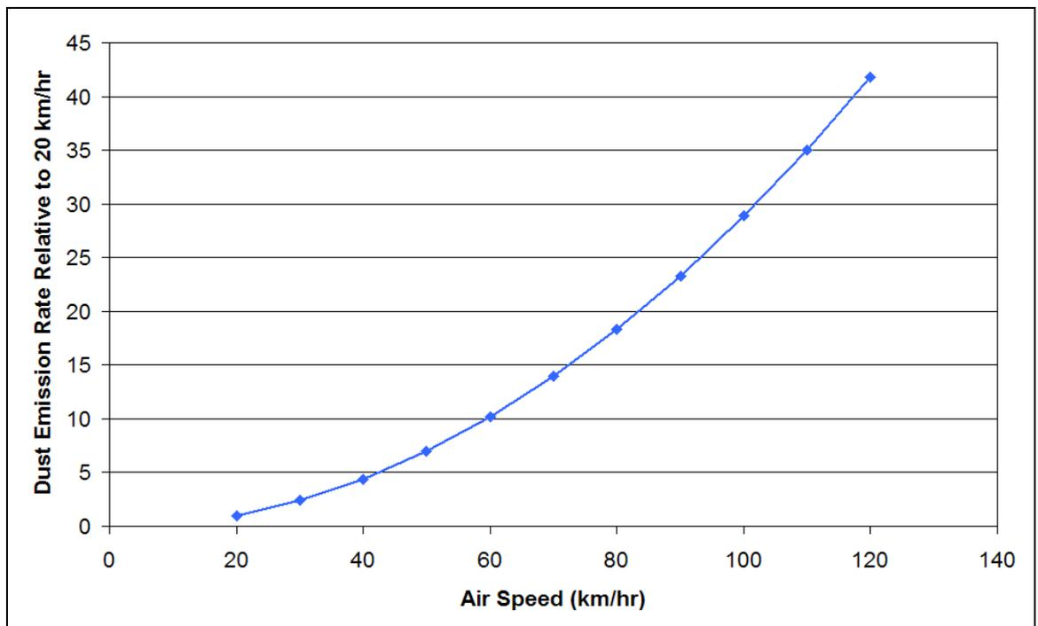
Figure 5.1 Dust emission rate due to airflow across an erodable surface based on Witt et al (1999)
