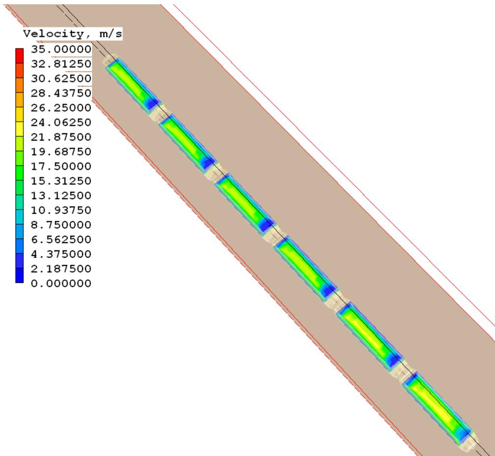
Figure 6.1.2b Model 1 – Unmodified wagon and single mound coal configuration contour coal surface velocity
