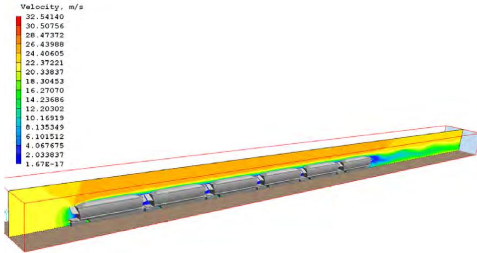
Figure 6.1.1h Model 6 – Unmodified wagon and Tee Pee Load mound coal configuration velocity contour isometric
