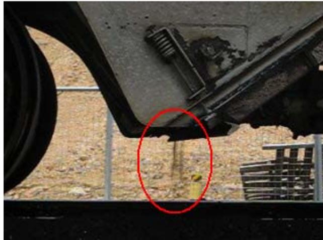
**Figure 4.2** Photograph showing an example of coal leaking from Kwik-Drop doors (Photograph taken by Simon Welchman on 15 November 2007 at DBCT rail loop on Goonyella System)
