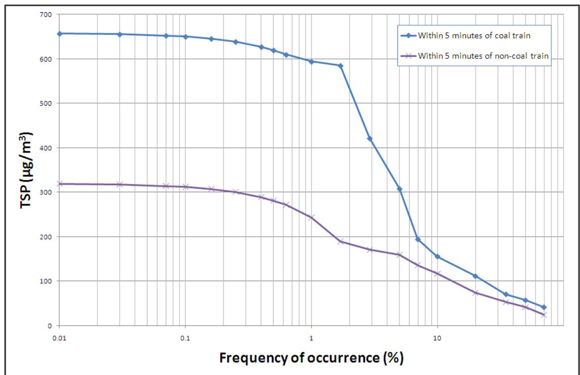
**Figure 7.10 Cumulative frequency distributions of 5-minute average concentrations of TSP ( $\mu\text{g}/\text{m}^3$ ) measured at about 10 metres from the edge of tracks at Raglan and filtered for type of train passing.**
