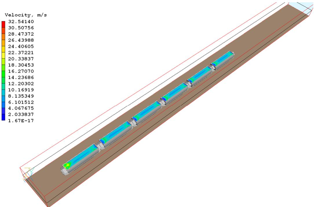
Figure 6.1.1i Model 6 – Unmodified Wagon and Tee Pee Load coal configuration velocity contour coal surface velocity
