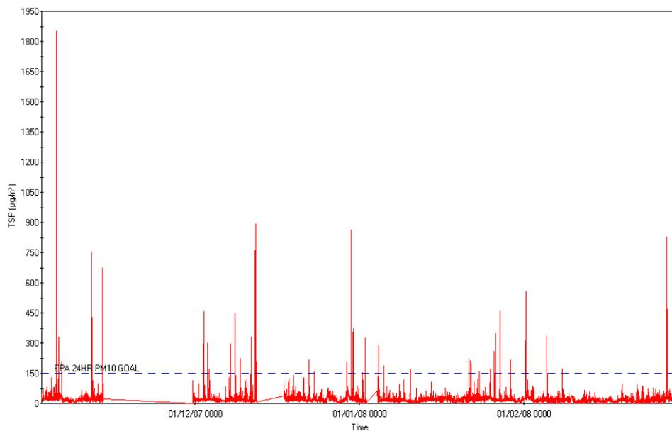
Figure 21. 5-minute average Concentration of TSP ( $\mu\text{g}/\text{m}^3$ ) measured at 10 metres from the tracks at Praguelds (November 11 2007 to February 29 2008)
