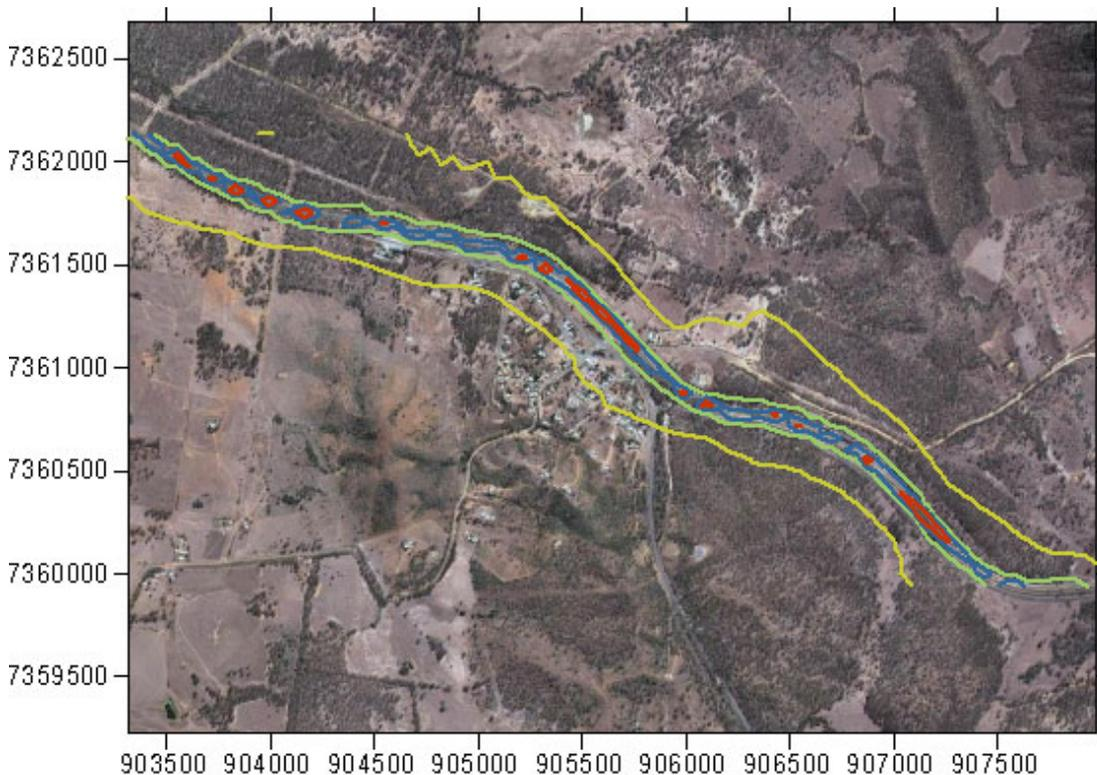
Figure 7.15 Scenario 2. Predicted maximum 24-hour average ground-level concentration of TSP ( $\mu\text{g}/\text{m}^3$ ) due to 2006/07 train movements on the Blackwater System. Train speed is 80 km/hr. The yellow line represents TSP concentration of 10  $\mu\text{g}/\text{m}^3$ , green 30  $\mu\text{g}/\text{m}^3$ , blue 50  $\mu\text{g}/\text{m}^3$  and red 70  $\mu\text{g}/\text{m}^3$ .
