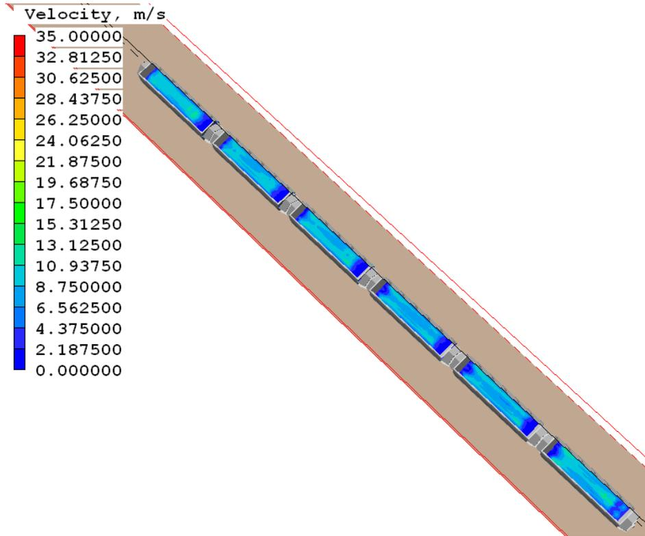
Figure 6.1.1b Model 1 – Unmodified wagon and single mound coal configuration contour coal surface velocity
