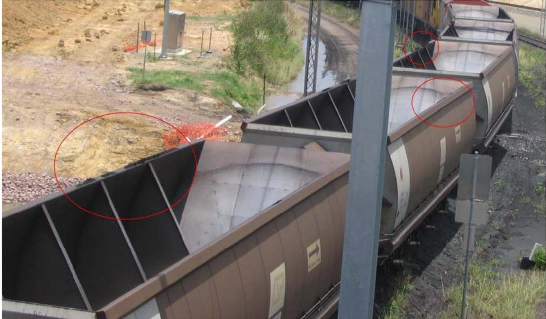
Figure 4.3 Photograph showing an example of coal on sills (Photograph taken by Simon Welchman on 15 November 2007 at DBCT rail loop on Goonyella System)
