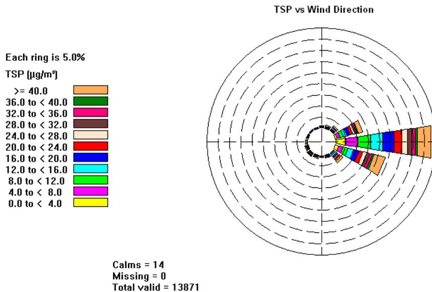
Figure 18. Wind rose of 5-minute average wind speed (m/s) and wind direction measured at 10 metres from the tracks at Boonal (December 31 2007 to March 6 2008). The directional spread of the columns indicates a predominance of East wind components; the coloured portion of the columns is TSP concentration
