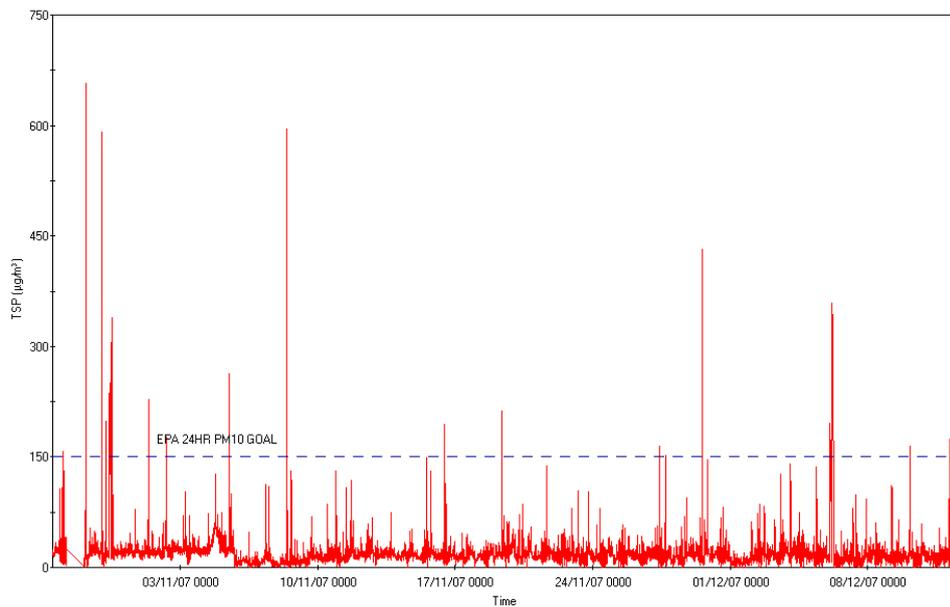
Figure 12. 5-minute average Concentration of TSP ( $\mu\text{g}/\text{m}^3$ ) measured at 10 metres from the tracks at Raglan (October 22 to December 13 2007)
