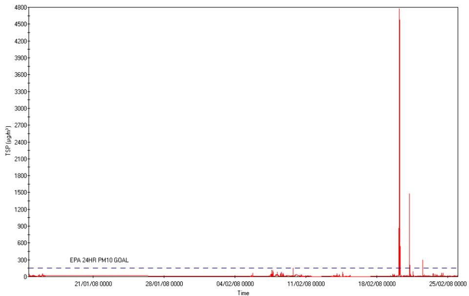
Figure 25. 5-minute average Concentration of TSP ( $\mu\text{g}/\text{m}^3$ ) measured at 10 metres from the tracks at Mindi (January 14 to February 26 2008)
