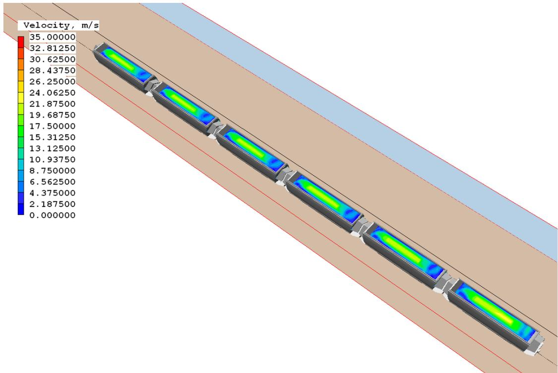
Figure 6.1.2f Model 3 – Wagon with 300 mm hungry board and single mound coal configuration velocity contour coal surface velocity
