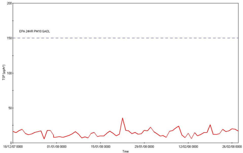
Figure 8. 24 hour average Mass Concentration of TSP ( $\mu\text{g}/\text{m}^3$ ) measured at 10 metres from the tracks at Earlsfield (December 18 2007 to February 29 2008)
