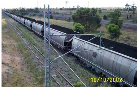
Figure 5 – Consistent Coal Profile
