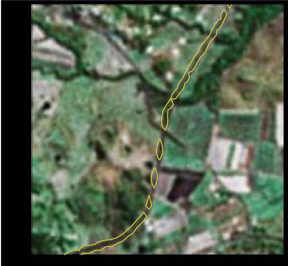
Figure 7.13 Scenario 1 (expanded version of Figure 7.12). Predicted maximum 24-hour average ground level concentration of TSP ( $\mu\text{g}/\text{m}^3$ ) due to 2006/07 train movements on the Goonyella system. Train speed is 38 km/hr. The yellow line represents TSP concentration of  $10 \mu\text{g}/\text{m}^3$ .
