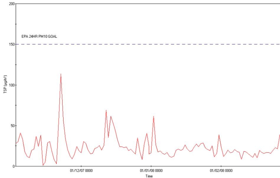
Figure 22. 24 hour average Concentration of TSP ( $\mu\text{g}/\text{m}^3$ ) measured at 10 metres from the tracks at Praguelds (November 11 2007 to February 29 2008)
