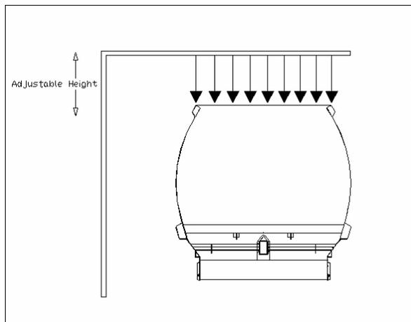
Figure 7 –Internal nozzles – water method
