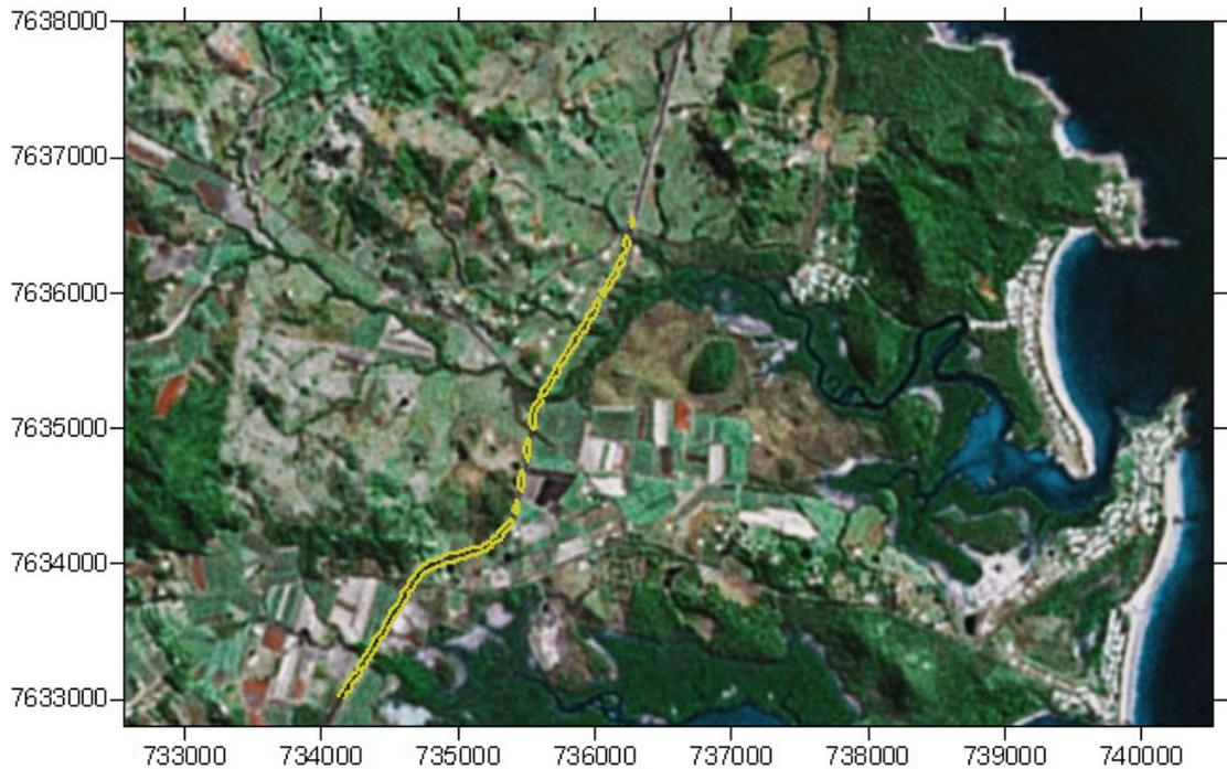
**Figure 7.12 Scenario 1. Predicted maximum 24-hour average ground level concentration of TSP (µg/m<sup>3</sup>) due to 2006/07 train movements on the Goonyella system. Train speed is 38 km/hr. The yellow line represents TSP concentration of 10 µg/m<sup>3</sup>.**
