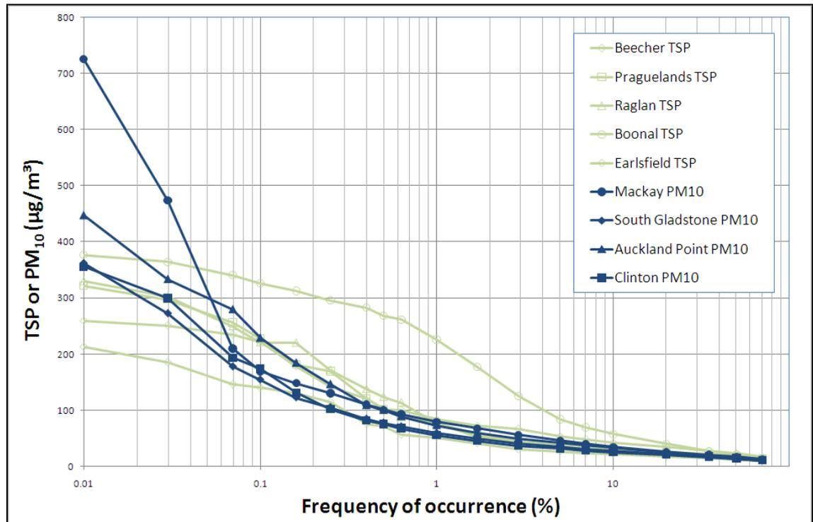
Figure 7.11 Cumulative frequency distributions of 1-hour average concentrations of TSP or PM<sub>10</sub> (µg/m<sup>3</sup>) measured during the Environmental Evaluation and compared with data from the EPA's sites at Mackay and Gladstone (South Gladstone and Clinton) and CQPA's monitoring site at Auckland Point.
