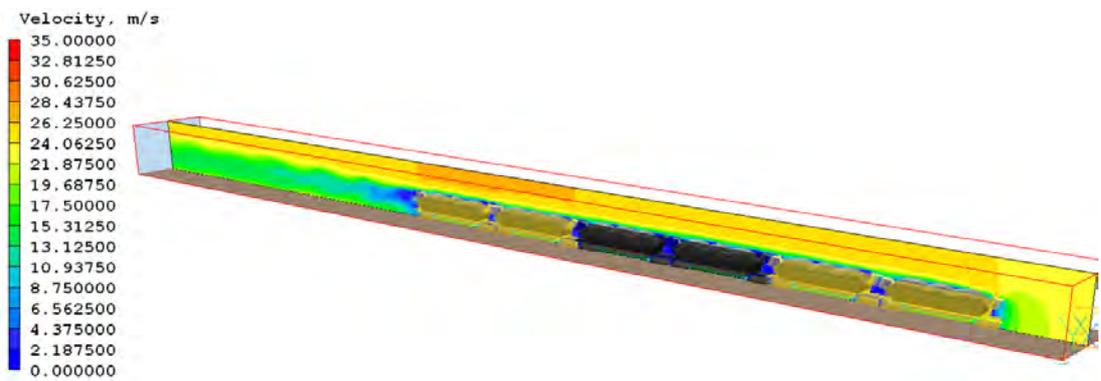
Figure 6.1.1c Model 2 – Unmodified wagon and three mound coal configuration velocity contour isometric
