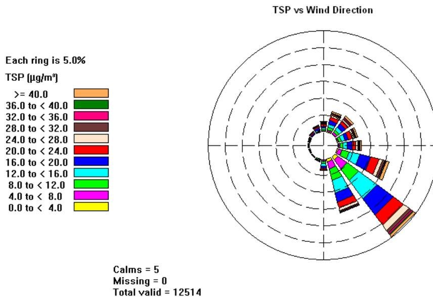
Figure 14. Wind/Dust rose of 5-minute average wind speed (m/s) and wind direction measured at 10 metres from the tracks at Raglan (October 22 to December 13 2007). The directional spread of the columns indicates a predominance South East wind components; the coloured portion of the columns is TSP concentration
