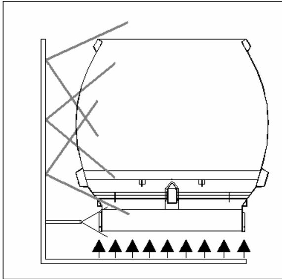
Figure 8 –External nozzles – water method
