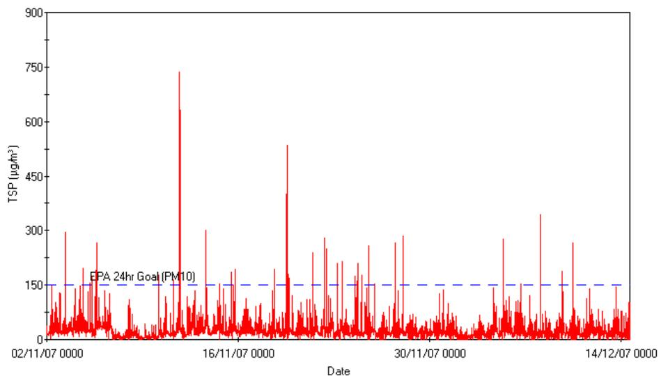
Figure 3. 5-minute average Mass Concentration of TSP ( $\mu\text{g}/\text{m}^3$ ) measured at 10 metres from the tracks at Beecher (November 11 to December 13 2007)
