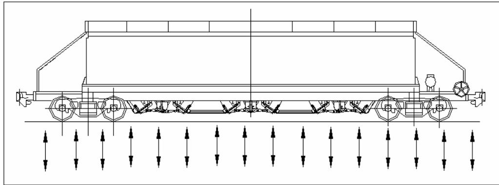
Figure 12 – Shock loading method
