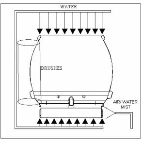
Figure 10 - Air / Water / Brush Combination Method
