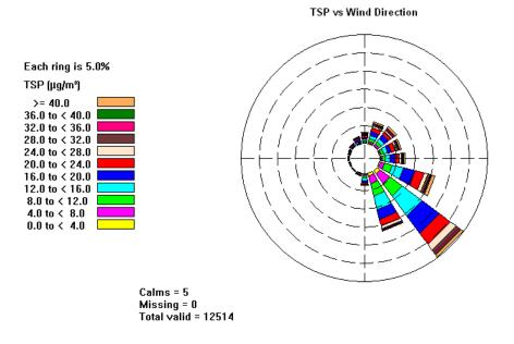
Figure 14. Wind/Dust rose of 5-mintue average wind speed (m/s) and wind direction measured at 10 metres from the tracks at Raglan (October22 to December 13 2007). The directional spread of the columns indicates a predominance South East wind components; the coloured portion of the columns is TSP concentration
