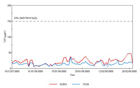
Figure 37. 24 hour average Concentration of TSP (µg/m<sup>3</sup>) measured at 10 metres from the tracks at Earlsfield for the time period December 18 2007 to February 29 2008. The blue line represents the TEOM and the red line is the Osiris
