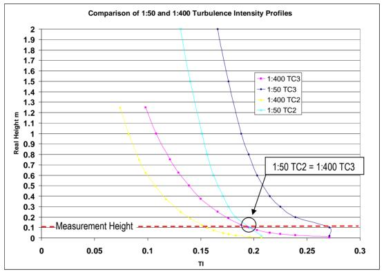
Figure 8 Turbulence Intensity Profiles (Source: AS1170.2)
