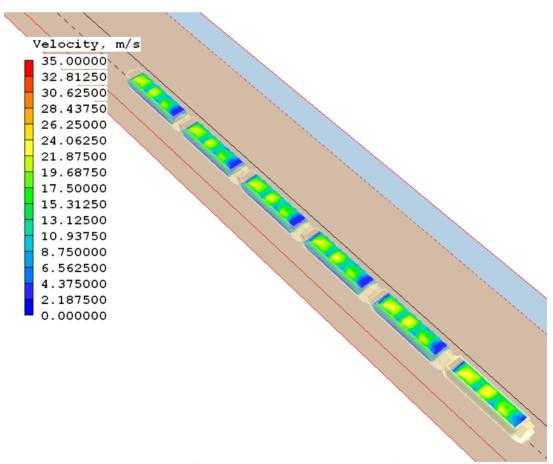
Figure 6.1.2d Model 2 – Unmodified wagon and three mound coal configuration velocity contour coal surface velocity
