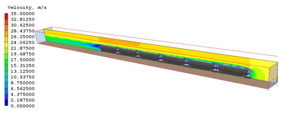
Figure 6.1.1e Model 3 – Wagon with 300 mm hungry board and three mound coal configuration velocity contour isometric
