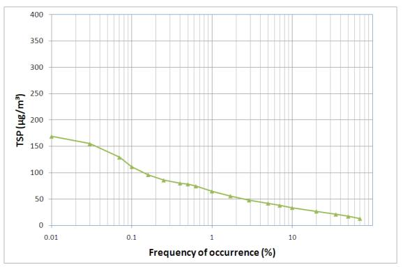
Figure 7.8 Cumulative frequency distributions of 1-hour average concentrations of TSP (µg/m<sup>3</sup>) measured at about 10 metres from the edge of tracks at Callemondah from April to October 2007.
