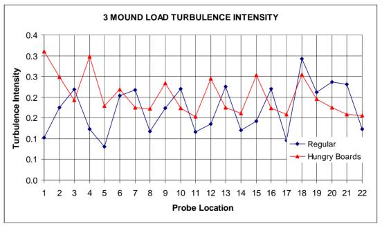
Figure 6.2.1d Turbulence intensity profile – 3 mound case
