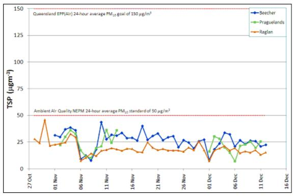
Figure 7.6 24-hour average Concentration of TSP (µg/m<sup>3</sup>) measured at about 10 metres from the tracks at Beecher, Praguelands and Raglan (October to 11 December 2007).
