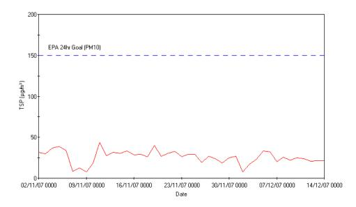
Figure 4. 24 hour average Mass Concentration of TSP (µg/m<sup>3</sup>) measured at 10 metres from the tracks at Beecher (November 11 to December 13 2007)
