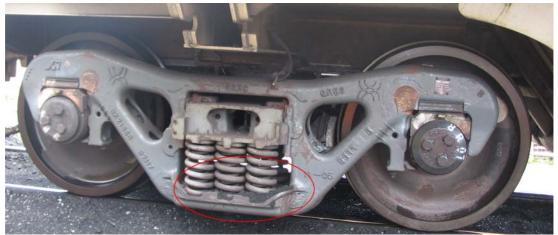
Figure 4.4 Photograph showing an example of coal on bogies (Photograph taken by Simon Welchman on 15 November 2007 at DBCT rail loop on Goonyella System)
