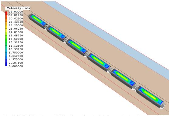
Figure 6.1.2f Model 3 – Wagon with 300 mm hungry baord and single mound coal configuration velocity contour coal surface velocity
