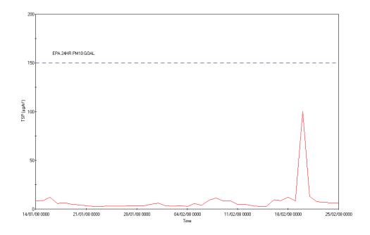
Figure 27. 24 hour average Concentration of PM10 (µg/m<sup>3</sup>) measured at 10 metres from the tracks at Mindi (January 14 to February 26 2008)
