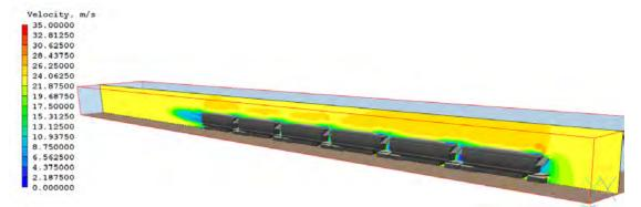
Figure 6.1.2e Model 3 – Wagon with 300 mm hungry baord and single mound coal configuration velocity contour isometric
