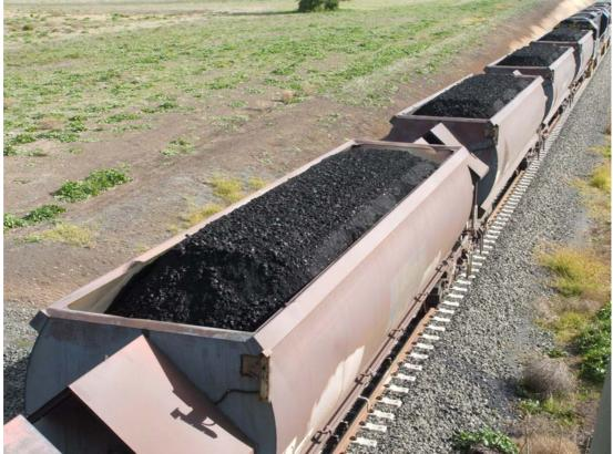
Figure 5.2 Photograph showing a 'garden bed' shape load profile (Photograph taken by Jim Harrison at Boggabri Coal on 13 July 2007)
