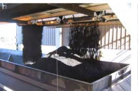
Figure 3 – Clamshell Transfer System
