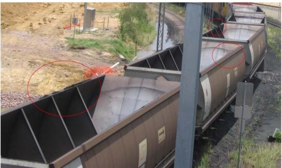
Figure 4.3 Photograph showing an example of coal on sills (Photograph taken by Simon Welchman on 15 November 2007 at DBCT rail loop on Goonyella System)
