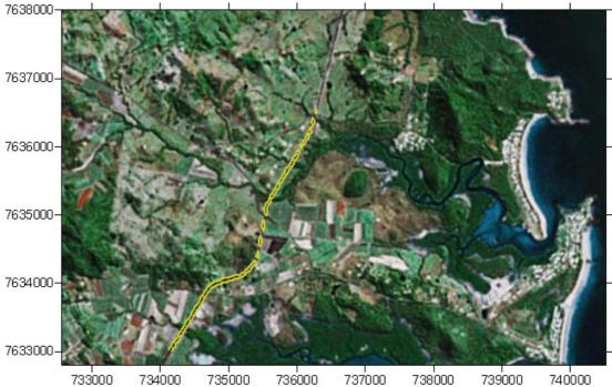
Figure 7.12 Scenario 1. Predicted maximum 24-hour average ground level concentration of TSP (μg/m<sup>3</sup>) due to 2006/07 train movements on the Goonyella system. Train speed is 38 km/hr. The yellow line represents TSP concentration of 10 μg/m<sup>3</sup>.
