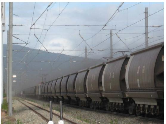
Figure 4.1 Photograph showing and example of coal dust emitted from the surface of coal wagons (Photograph taken by Jim Harrison on 15 December 2007 at Nebo road turnoff on Goonyella System)
