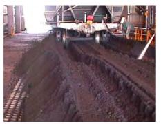
Figure 9 – Coal Ploughing Leading to a Derailment
