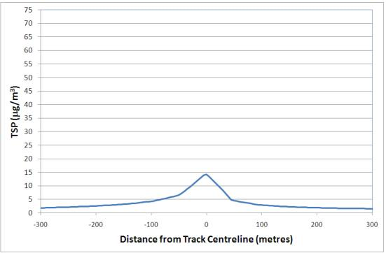
Figure 7.14 Scenario 1. Cross-section of predicted maximum 24-hour average ground level concentration of TSP (µg/m<sup>3</sup>) due to 2006/07 train movements on the Goonyella system. Train speed is 38 km/hr.
