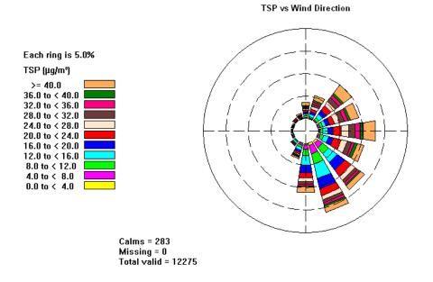
Figure 5. Wind/Dust rose of 5-mintue average wind direction and TSP (µg/m<sup>3</sup>) measured at 10 metres from the tracks at Beecher (November 11 to December 13 2007). The directional spread of the columns indicates a predominance of East to South East wind components; the coloured portion of the columns is TSP concentration
