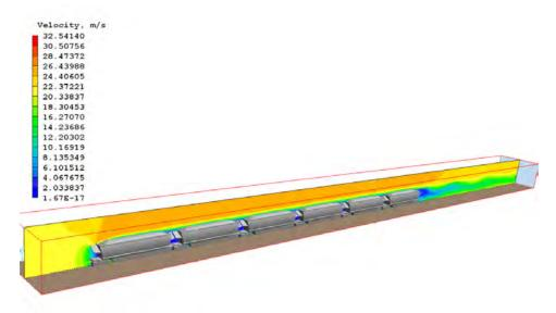
Figure 6.1.1h Model 6 – Unmodified wagon and Tee Pee Load mound coal configuration velocity contour isometric
