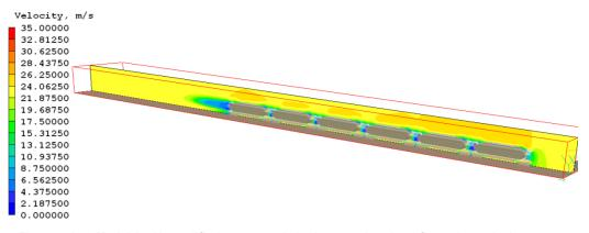
Figure 6.1.2a Model 1 – Unmodified wagon and single mound coal configuration velocity contour isometric
