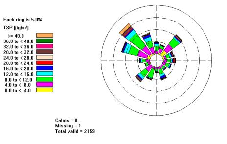
Figure 28. Wind/Dust rose of 5-mintue average wind speed (m/s) and wind direction measured at 10 metres from the tracks at Mindi (January 14 to February 26 2008). The directional spread of the columns indicates a predominance of North West wind components; the coloured portion of the columns is TSP concentration
