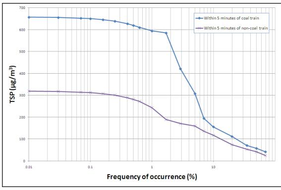
Figure 7.10 Cumulative frequency distributions of 5-minute average concentrations of TSP  $(\mu g/m^3)$  measured at about 10 metres from the edge of tracks at Raglan and filtered for type of train passing.
