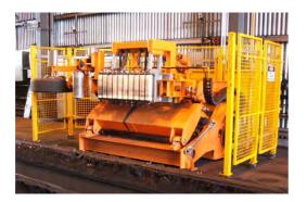
Figure 7 – Automatic Wagon Vibrator
