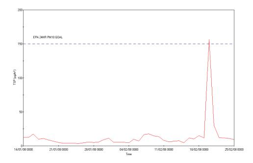
Figure 26. 24 hour average Concentration of TSP (µg/m<sup>3</sup>) measured at 10 metres from the tracks at Mindi (January 14 to February 26 2008)
