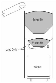
Figure 2 – Batch Weighing System
