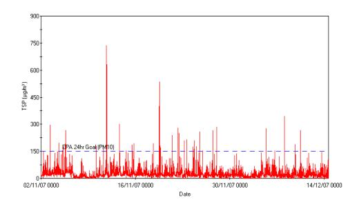
Figure 3. 5-minute average Mass Concentration of TSP (µg/m<sup>3</sup>) measured at 10 metres from the tracks at Beecher (November 11 to December 13 2007)
