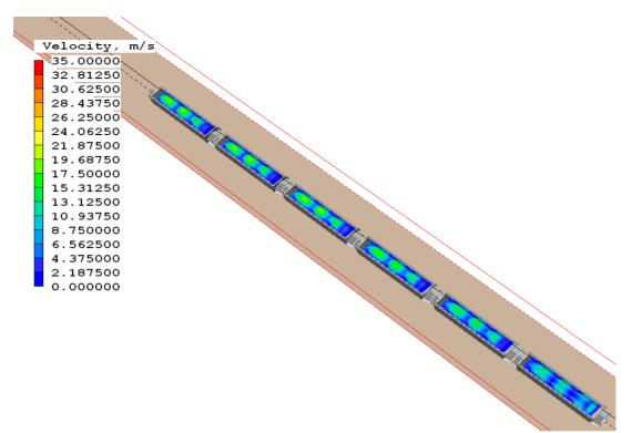
Figure 6.1.1f Model 3 – Wagon with 300 mm hungry board and three mound coal configuration velocity contour coal surface velocity
