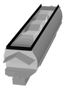
Figure 3 Isometric view of train with hungry board and three mound coal loading
