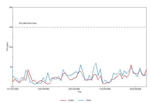
Figure 32. 24 hour average Concentration of TSP (µg/m<sup>3</sup>) measured at 10 metres from the tracks at Boonal for the time period December 31 2007 to March 6 2008. The blue line represents the TEOM and the red line is the Osiris
