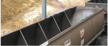
Figure 3 – Parasitic Load on Wagon Sills
