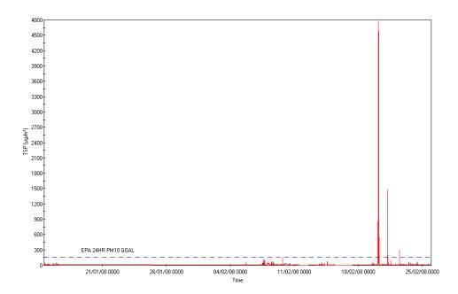
Figure 25. 5-minute average Concentration of TSP (µg/m<sup>3</sup>) measured at 10 metres from the tracks at Mindi (January 14 to February 26 2008)
