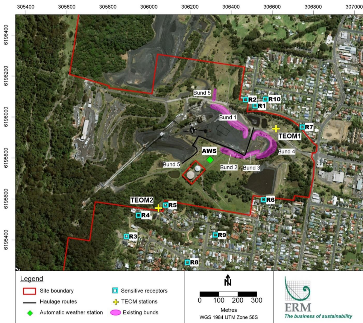
Figure 2.1 Existing site, proposed layout and dust monitoring sites
