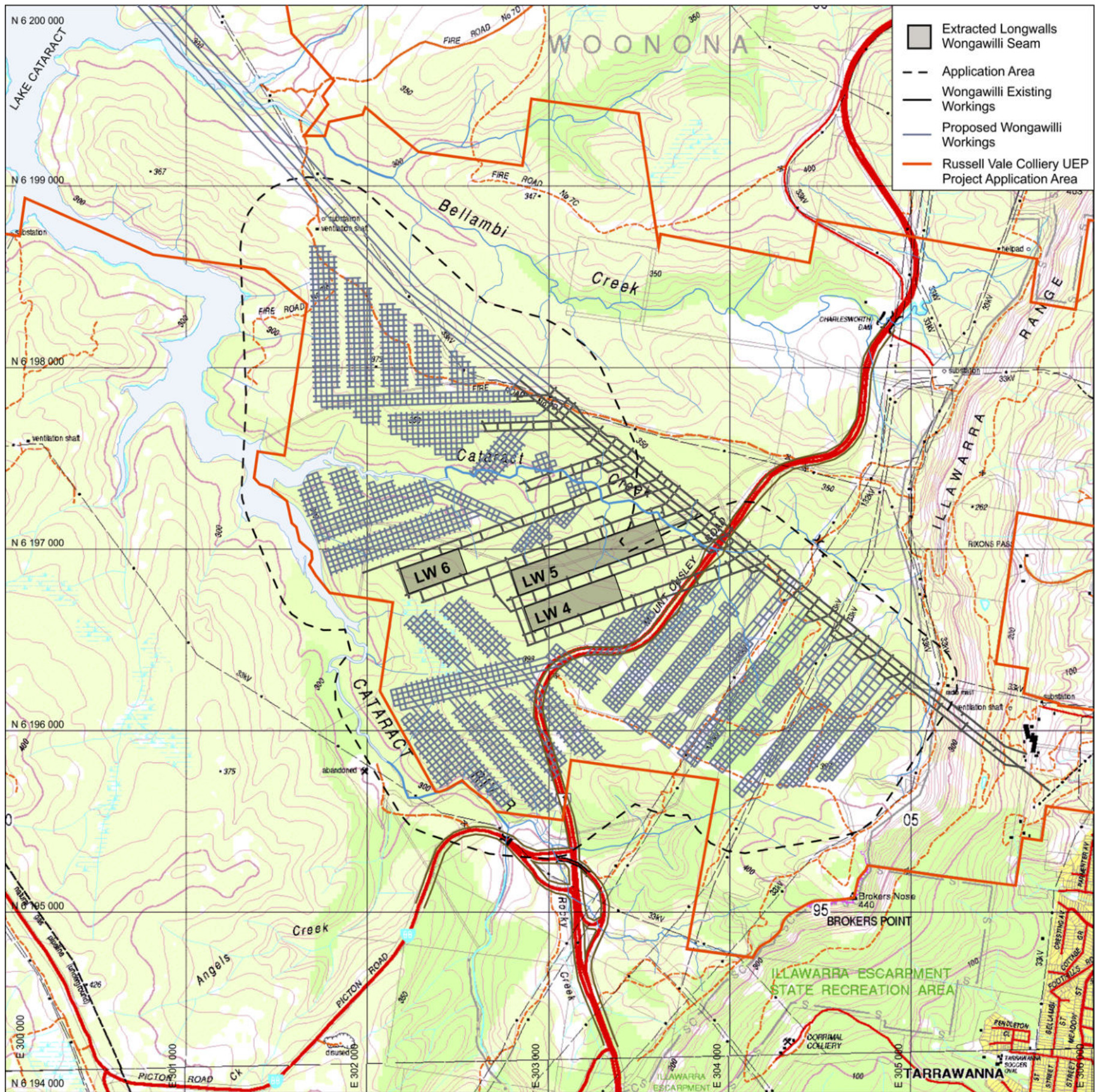
Figure 1: Plan showing location of Application Area with existing and proposed Wongawilli Seam proposed workings superimposed onto a 1:25,000 topographic series map with creek alignments update based on LiDAR imaging of the ground surface.
