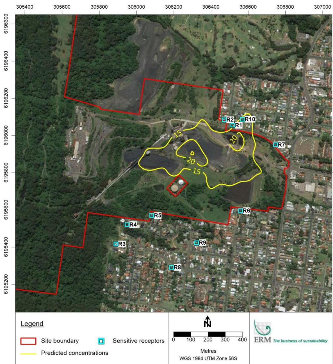
Figure 9: Predicted maximum 24-hour average PM 2.5 concentrations when the maximum production coincides with worst case dispersion conditions
