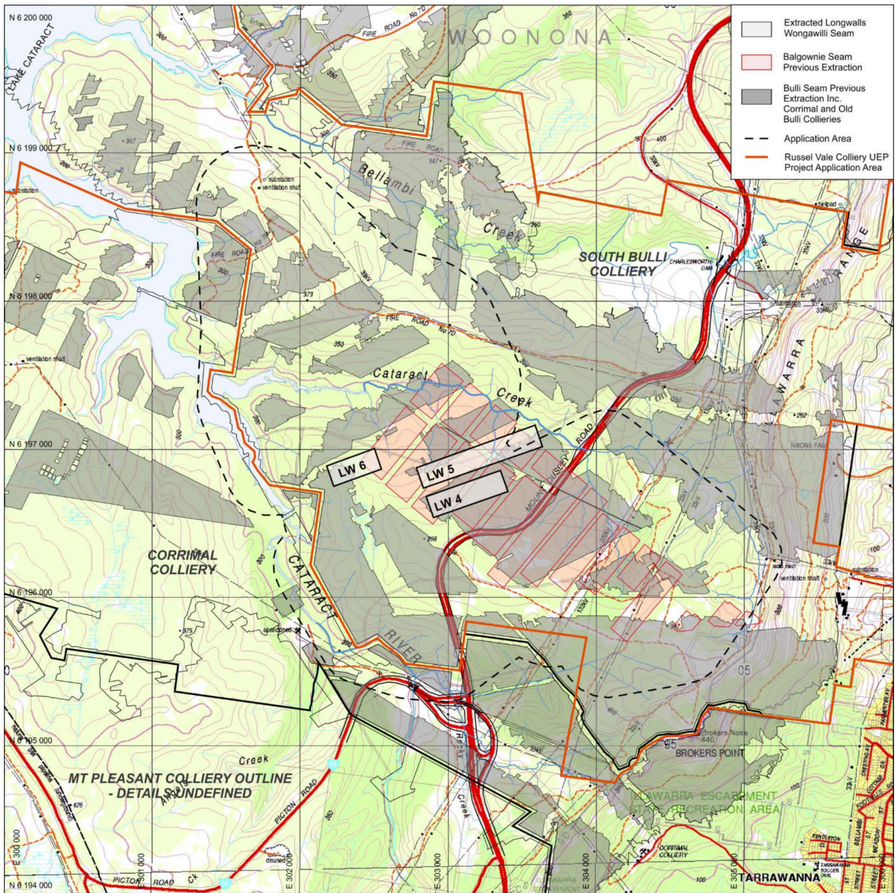
Figure 14: Plan showing extent of previous secondary extraction in Bulli Seam (black), Balgownie Seam (red) and Wongawilli Seam (grey) in the Application Area.
