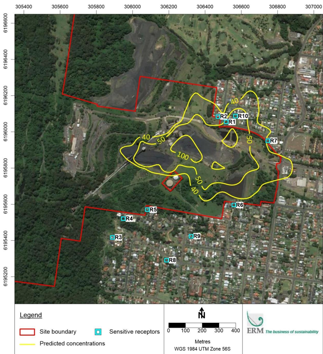
Figure 10: Predicted maximum 24-hour average PM_{10} concentrations when the maximum production coincides with worst case dispersion conditions
