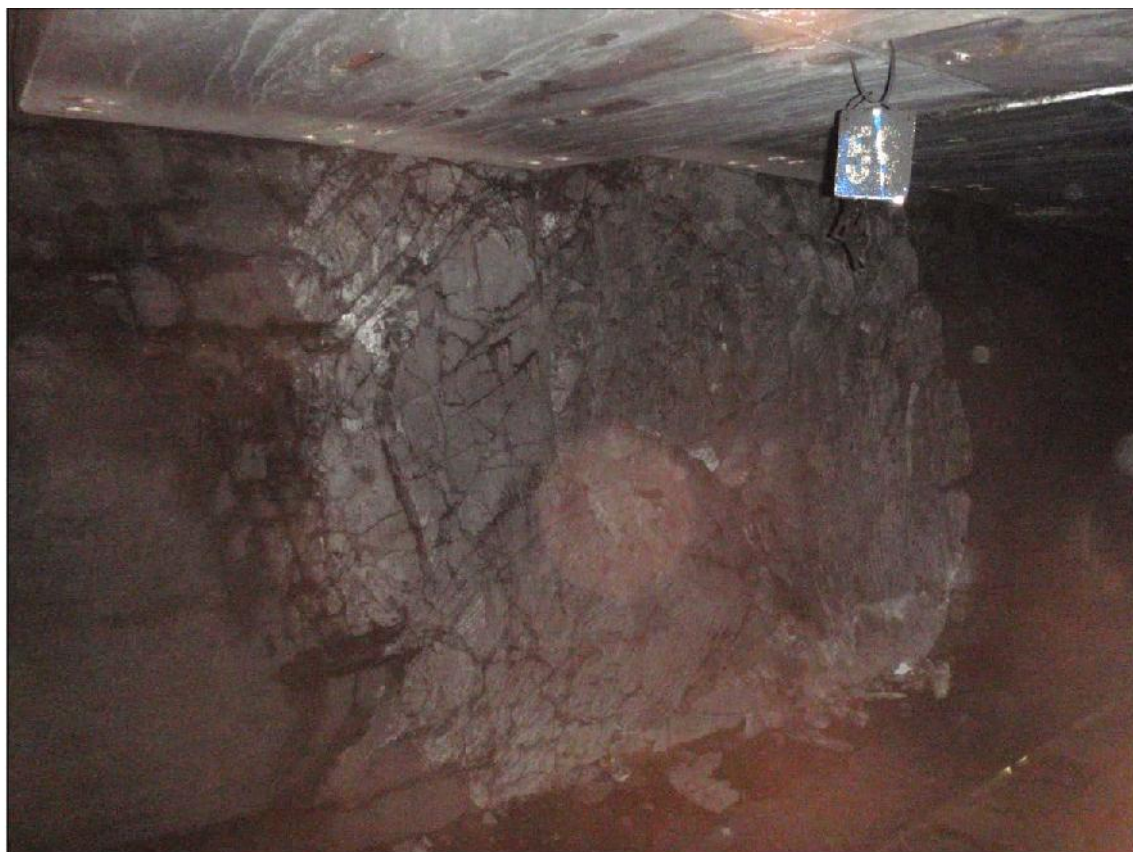
Figure 5: Photograph of Dyke D8 exposed underground in the longwall face of Longwall 5.
