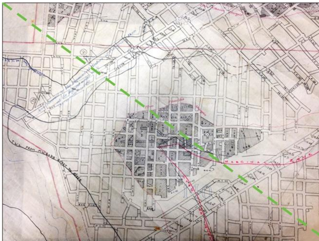
Figure 18: Shows a section of the Bulli Seam Record Tracing for South Bulli Colliery along the suggested projection (dotted line) of the Corrimal Fault below the Cataract Reservoir. The '5 Chains Margin' and 35° Angle of Draw (0.7D barrier) Marginal Zone is also shown. Reduced Levels are in feet on a datum 1000' below MWSDB standard datum.
