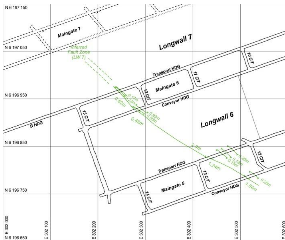
Figure 10: Detail of intersections of the Corrimal Fault in the Wongawilli Seam - Longwall 6 goaf omitted for clarity.
