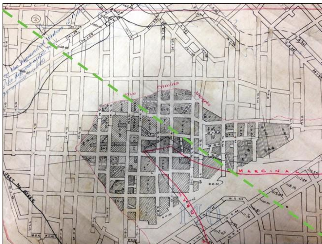
Figure 18: Shows a section of the Bulli Seam Record Tracing for South Bulli Colliery along the suggested projection (dotted line) of the Corrimal Fault below the Cataract Reservoir. The '5 Chains Margin' and 35° Angle of Draw (0.7D barrier) Marginal Zone is also shown. Reduced Levels are in feet on a datum 1000' below MWSDB standard datum.
