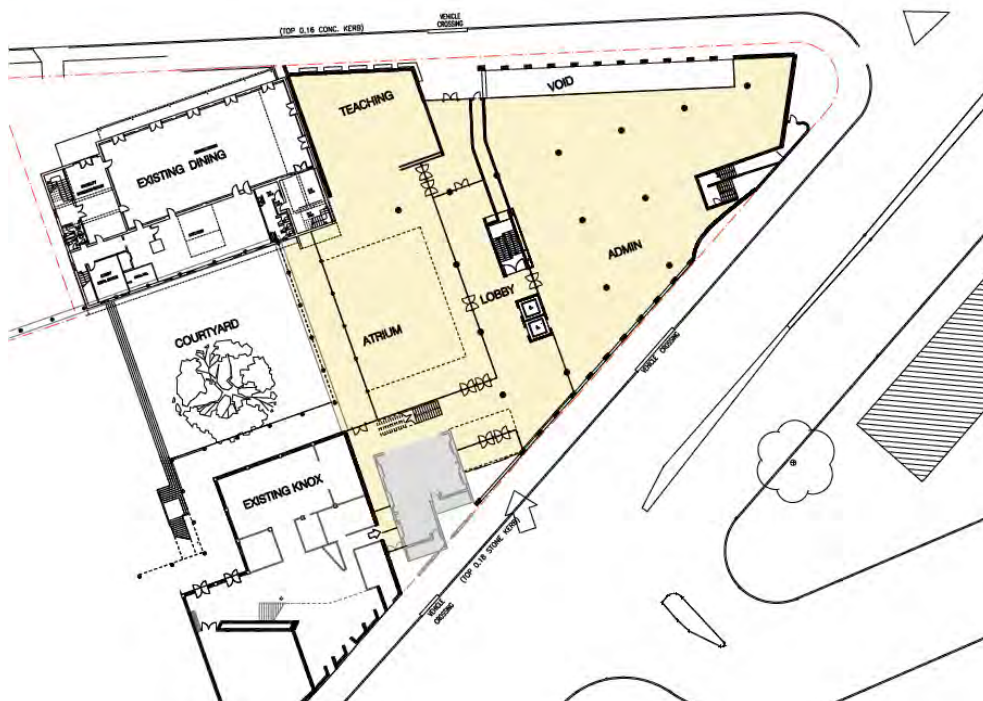
Figure 2: Ground Level Plan of Library Building
