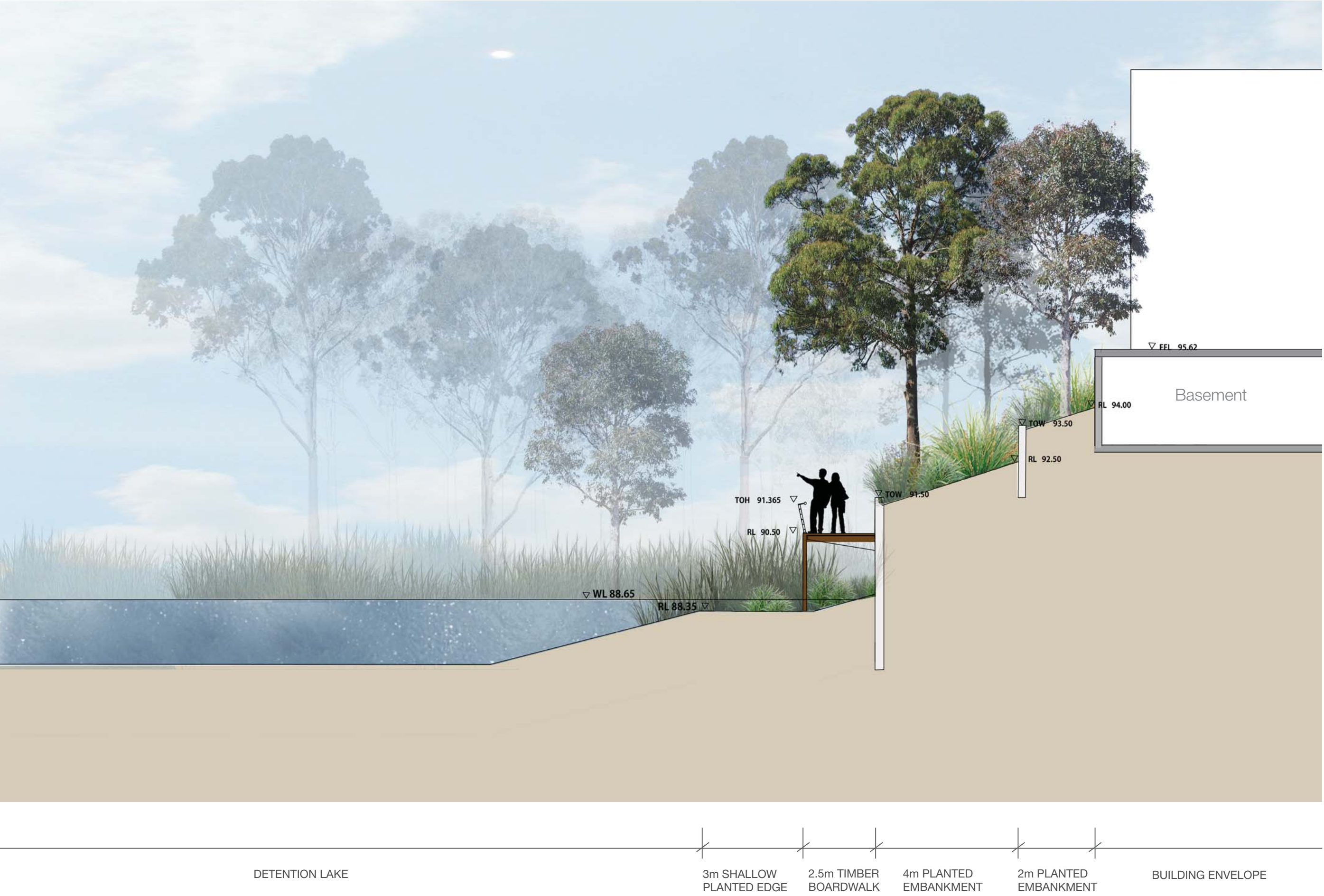
Section A-A Detention Lake interface Scale 1:100 @ A1
