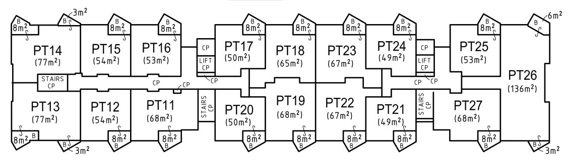
THESE PLANS HAVE BEEN BASED UPON THE ARCHITECTURAL PLANS PREPARED BY PTW ARCHITECTS. AREAS SHOWN HEREON HAVE BEEN DETERMINED FROM THESE PLANS AND ARE SUBJECT TO CONSTRUCTION AND FINAL SURVEY.
