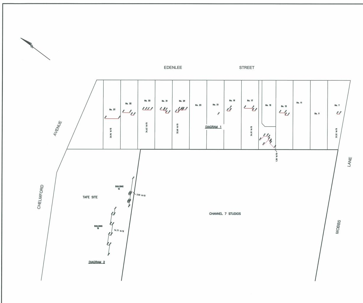
LEVELS ARE BASED ON AUSTRALIAN HEIGHT DATUM (AHD) USING SSM 91910 WITH RL OF 102.125m (ACC B) LOCATED AT EDENLEE AND DUNLOP STREETS
