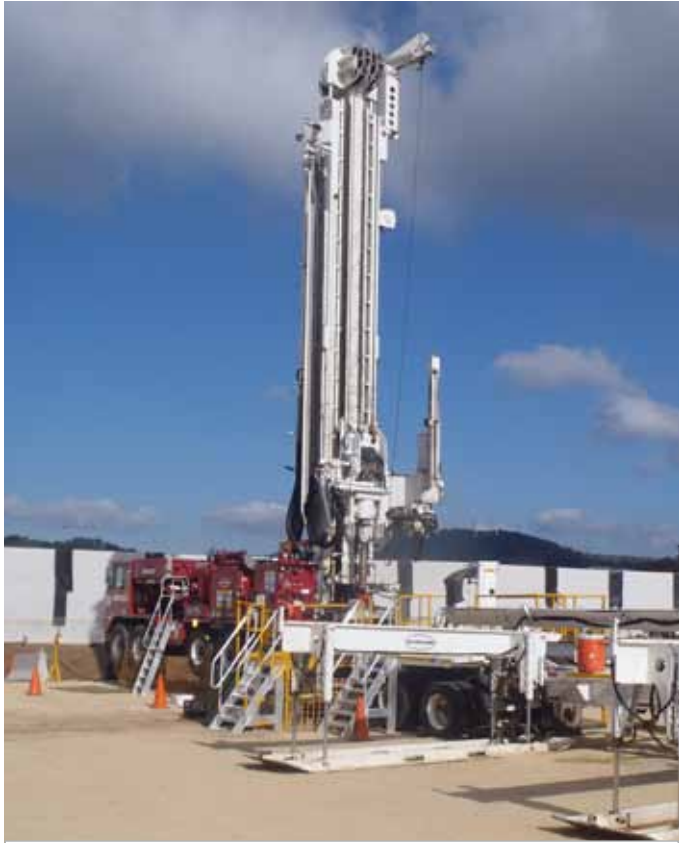
The medium radius drilling site is prepared using a drill rig that is positioned within a compound surrounded by sound barriers.
