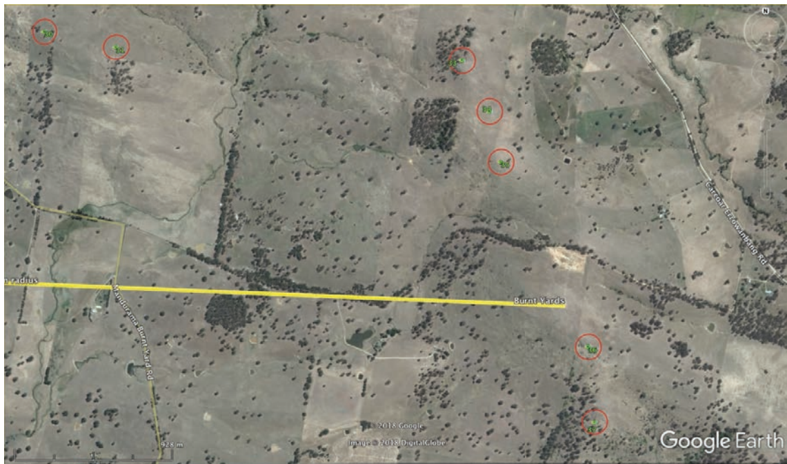
Figure 4-31 Path I - First Fresnel zone shown in yellow
