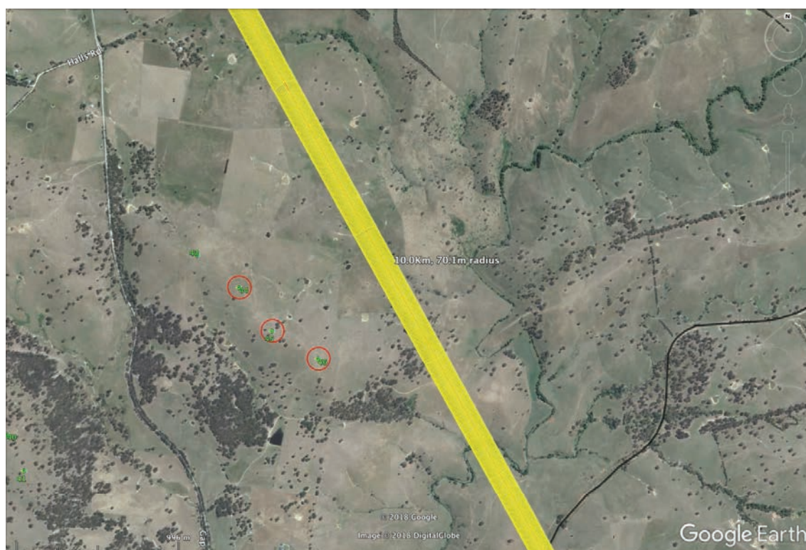
Figure 4-25 Path G - First Fresnel zone shown in yellow
