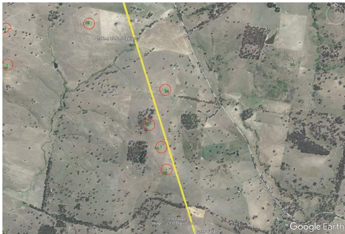
Figure 4-22 Path F - First Fresnel zone shown in yellow – southern portion
