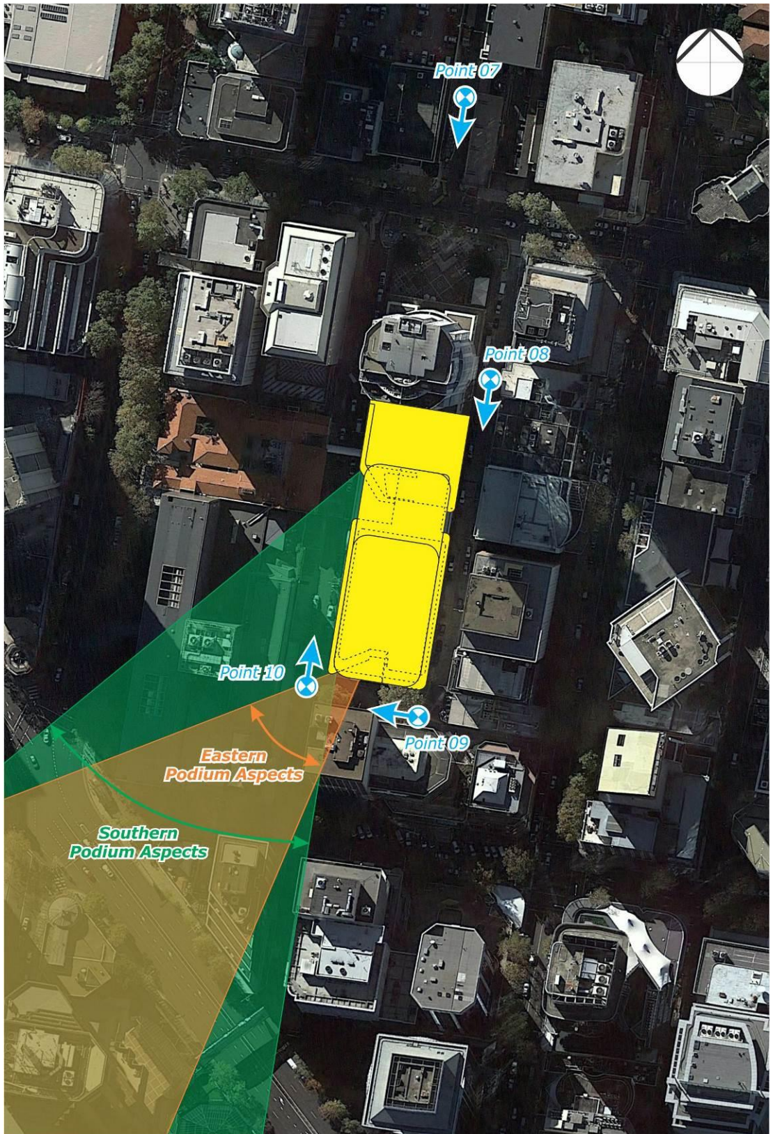
Figure 2b: Check Zones and Study Point Locations Unique Podium Level Façade Aspects (the check zones are the areas where glare could potentially be observed)
