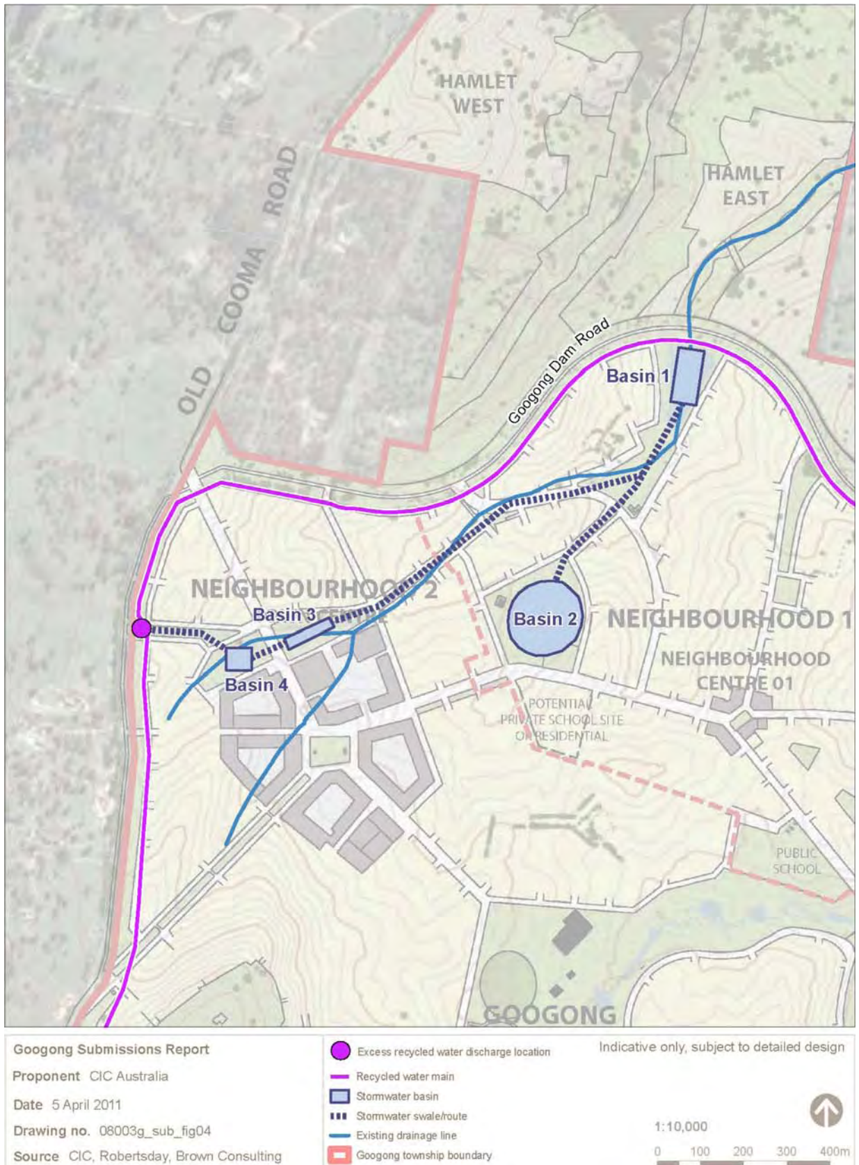
Figure 6: Proposed treated effluent discharge and stormwater system
