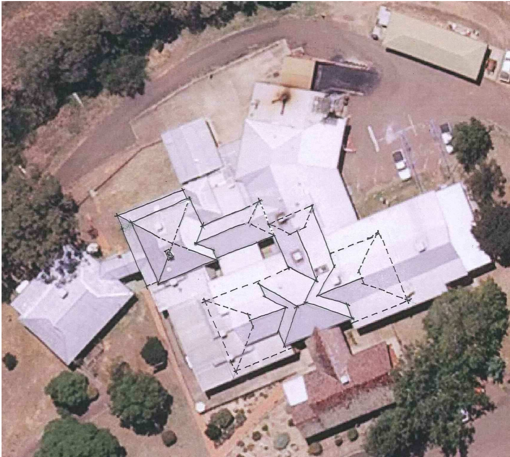
Plate 4.1: The outline of the roofs to the surviving original 1905 & 1909 buildings superimposed on a current aerial photograph of the hospital buildings. The dotted lines indicate the extent of the earlier roofs now enveloped in the present roof structure.
