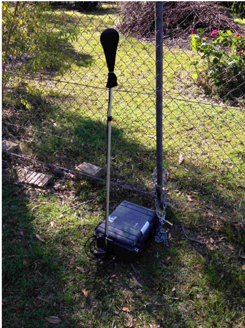
Figure 3 – Example unattended noise logger setup
