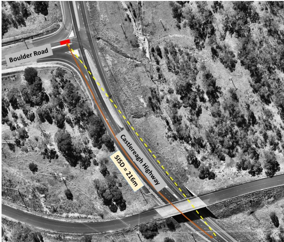
Figure 4-5 Sight Triangle for Truck Exiting Boulder Road - Mount Piper Power Station
