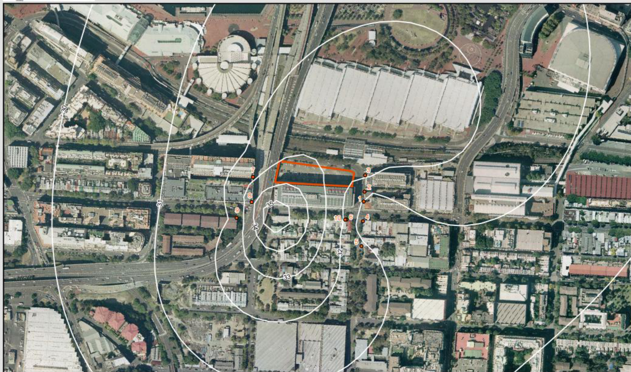
Figure 7-2: Maximum predicted annual ground level cumulative NO x (as NO 2 ) concentration ( \mu\text{g}/\text{m}^3 ) from the turbine units using the OLM approach
