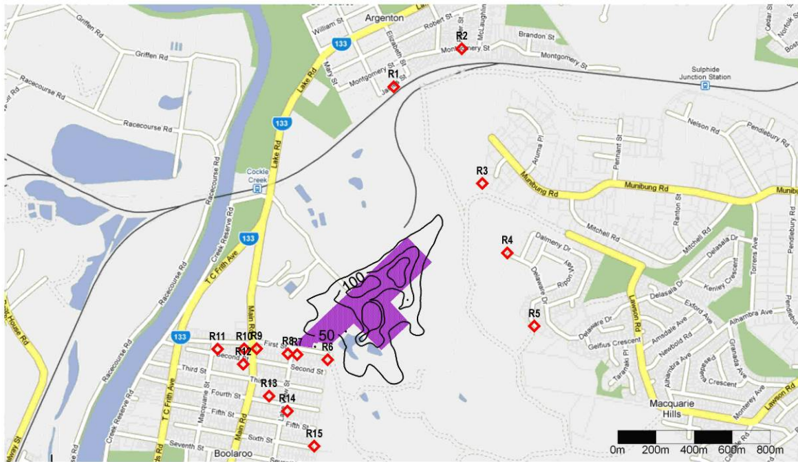
Maximum 24-hour Average PM10 ( \mu\text{g}/\text{m}^3 ) due to IPL Cockle Creek Remediation Concurrent Stages 2 to 4 Emissions
