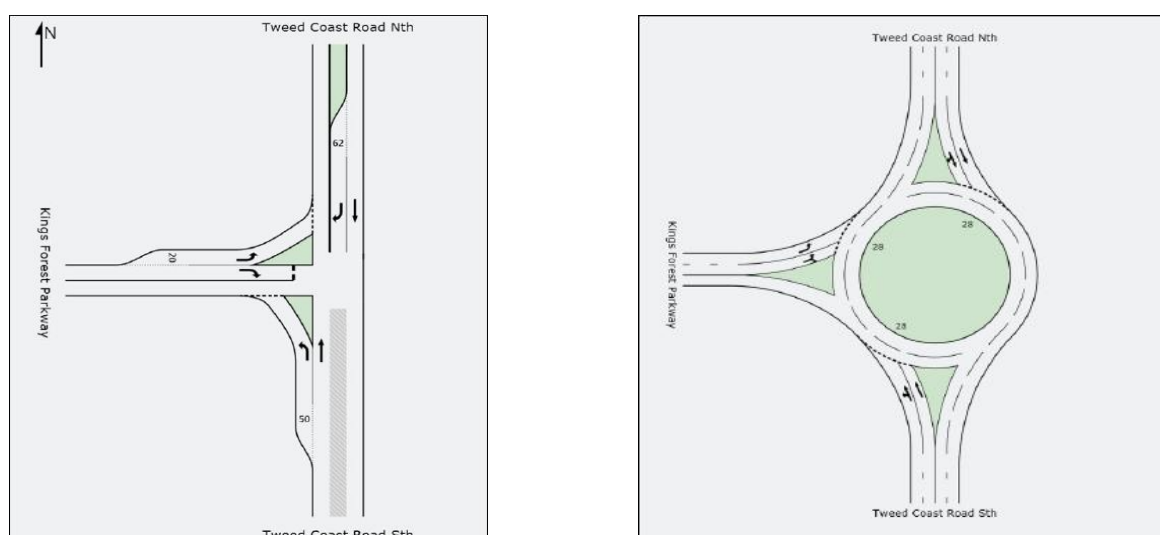
Figure 26: Interim and Ultimate Intersection Arrangements for Tweed Coast Road and Kings Forest Parkway
