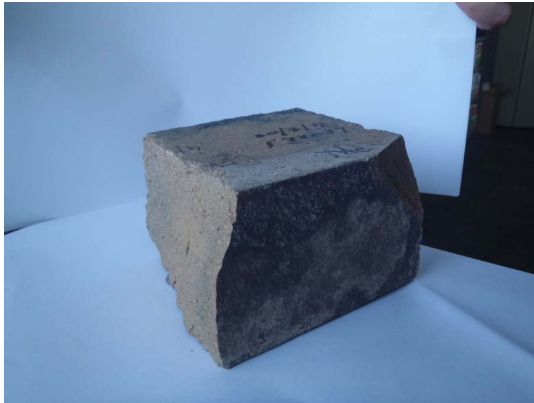
Exposed face of internal stack brick from level 1
