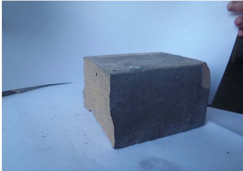
Exposed face of internal stack brick from level 15
