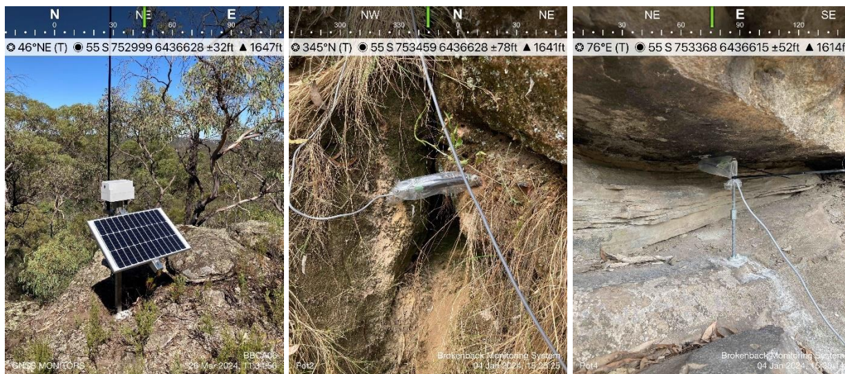
Photo 5 Example of a GNSS & Potentiometer Units within the BBCA
