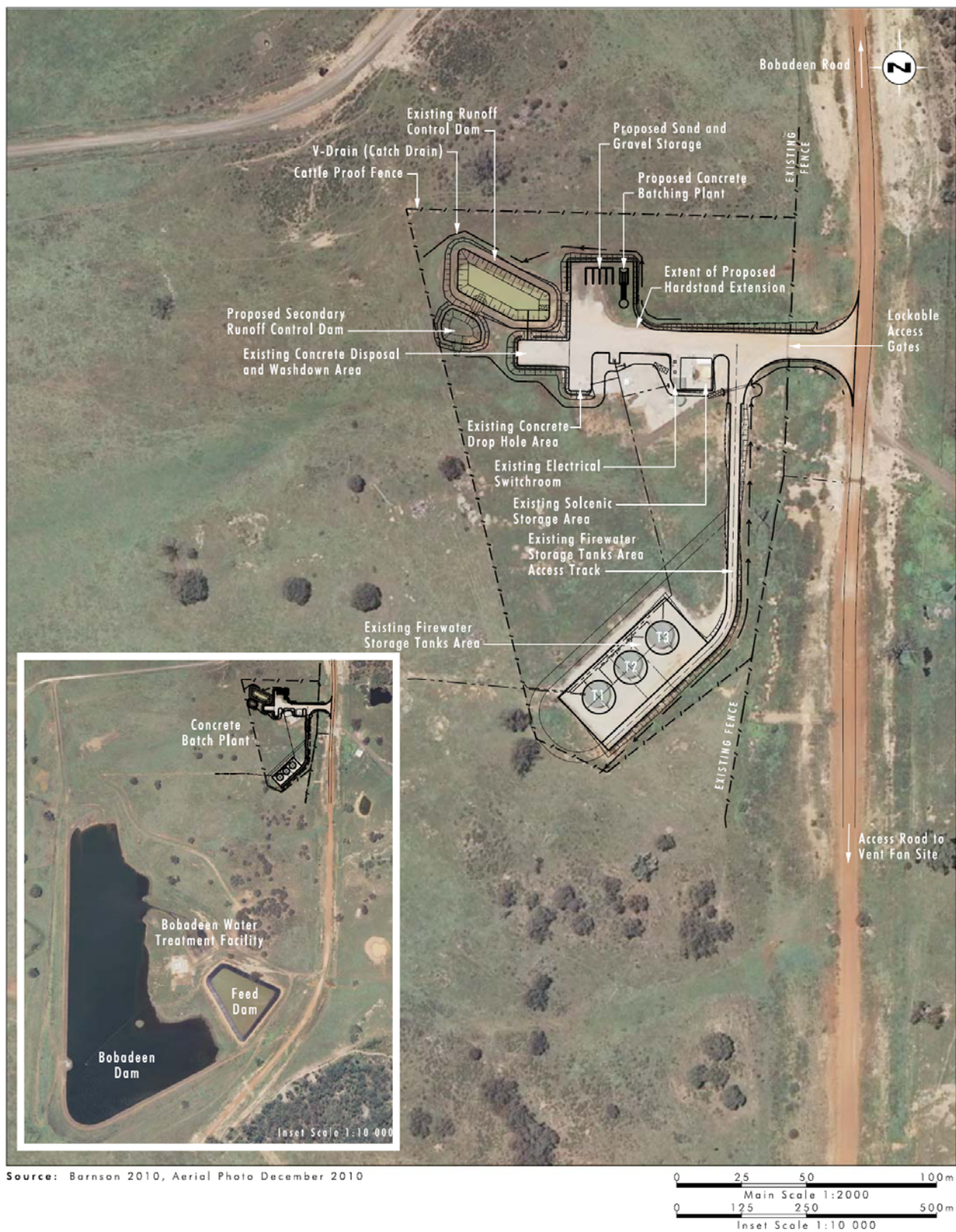
FIGURE 3.2 Proposed Concrete Batching Plant Site Layout
