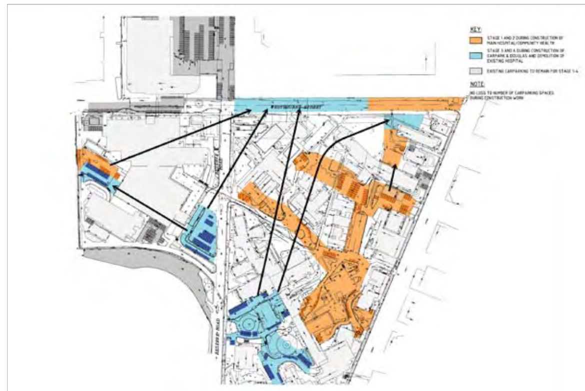
Figure 23: Carpark decanting during staged works, prepared by Hyder Consulting
