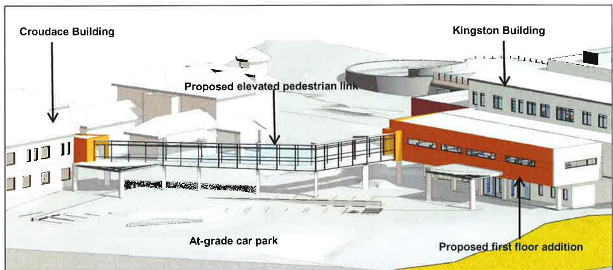
Figure 5: Perspective view showing the proposed link between the Kingston Building and Croudace Building (Source: Proponent)
