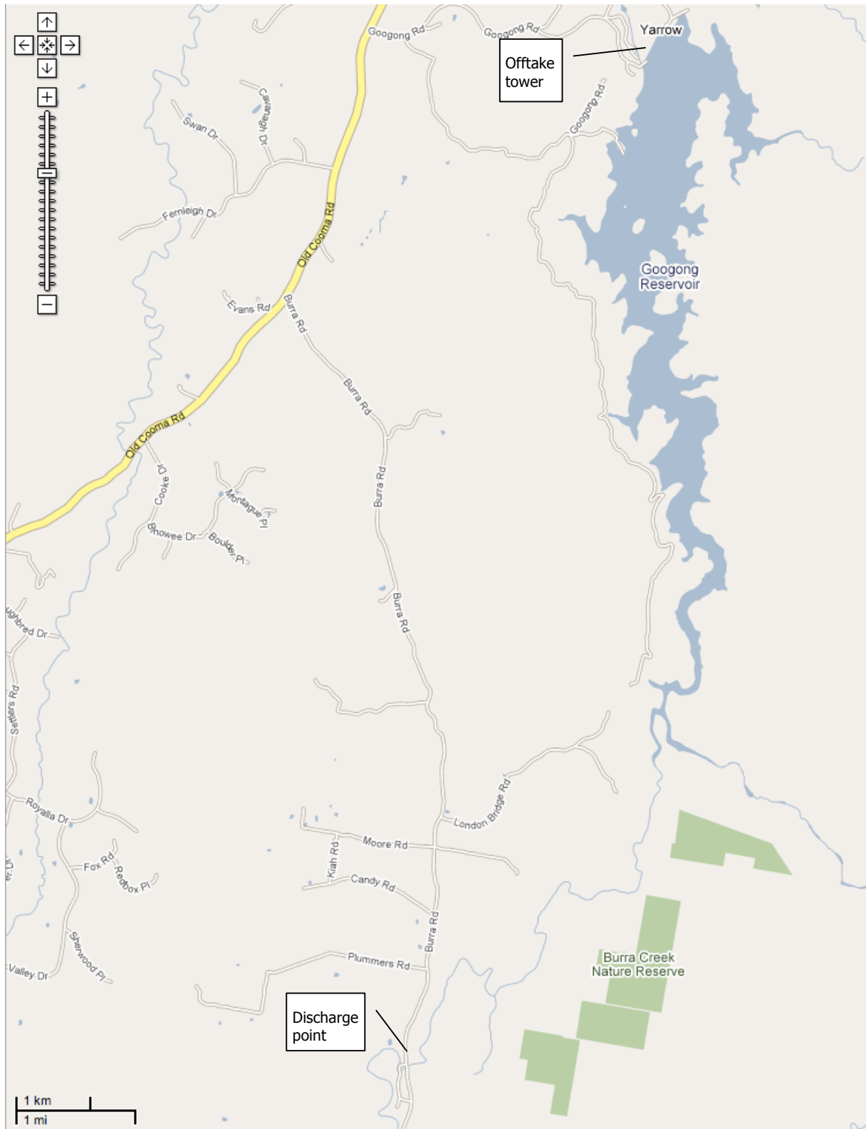
Figure 2-1. Map showing discharge point of the Murrumbidgee River source water into Burra Creek as well as the offtake tower that supplies water from the Googong Reservoir to the Googong Water Treatment Plant (base map: © Google maps).
