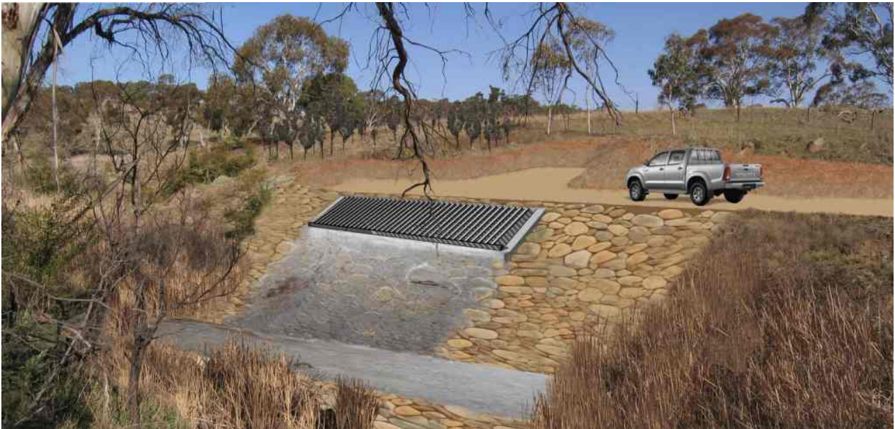
Figure 2.6 Visual representation of discharge structure
