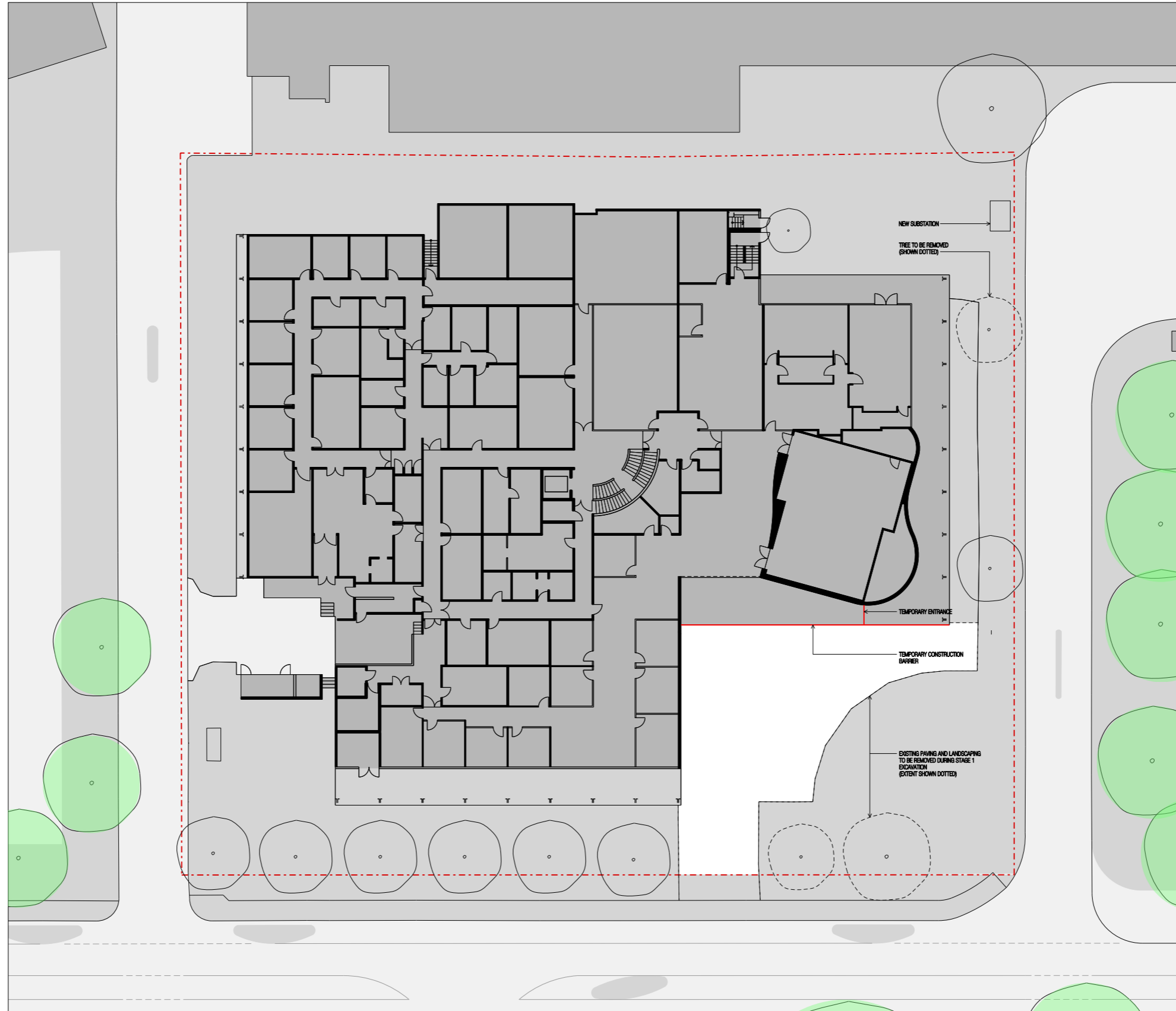
1 STAGE 1 DEMOLITION PLAN - GROUND FLOOR SCALE 1:200
