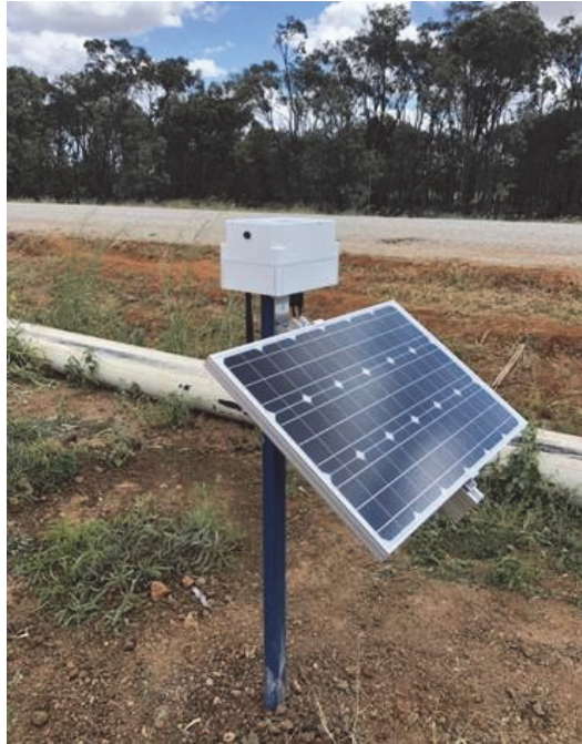
Fig. 6.5 Nominal GNSS unit installation set-up
